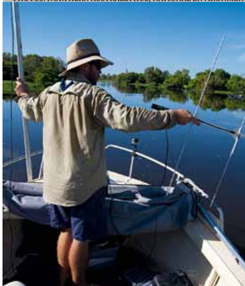
A directional antenna is used in boat surveys to detect where the tagged fish are within one metre, and an aerial is used in helicopter surveys to log the GPS coordinates of the fish.
