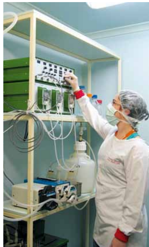
Pilot-scale production of Corrovac vaccine at the Fish Health Unit, Tasmanian DPIPWE, Launceston. The fermenter is used for mass culture of the Tasmanian Rickettsia -like organism.
