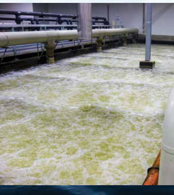
Above A recirculating aquaculture system at a Huon Aquaculture hatchery filters and treats water before it is reused in the fish grow-out tanks at the site.
