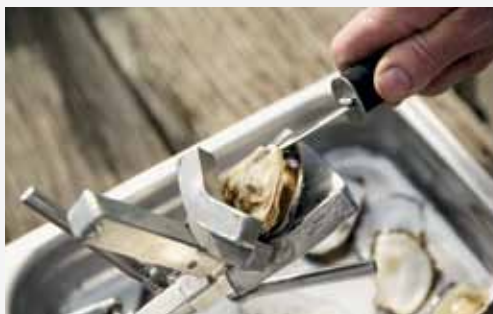
NSW fisher Steve Siminis has developed a new oyster shucking system that will make it easier to put fresh, premium oysters on the menu in more restaurants. The opening system provides a secure grip on the oysters, making them safer and easier to open.
