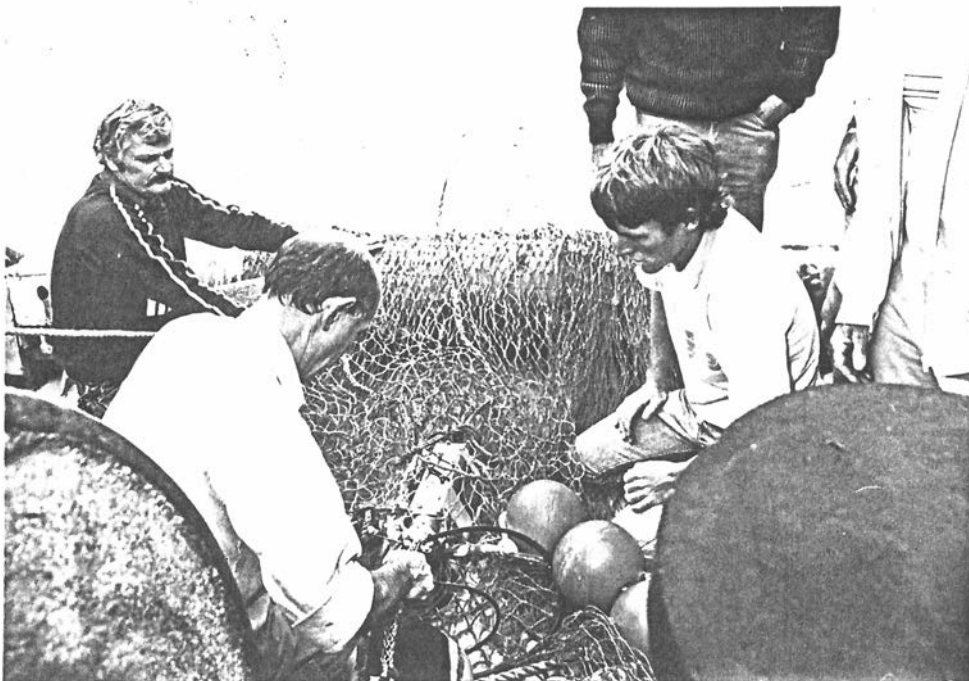
(4) Securing the netsounder transducers to headline of the trawl net.
