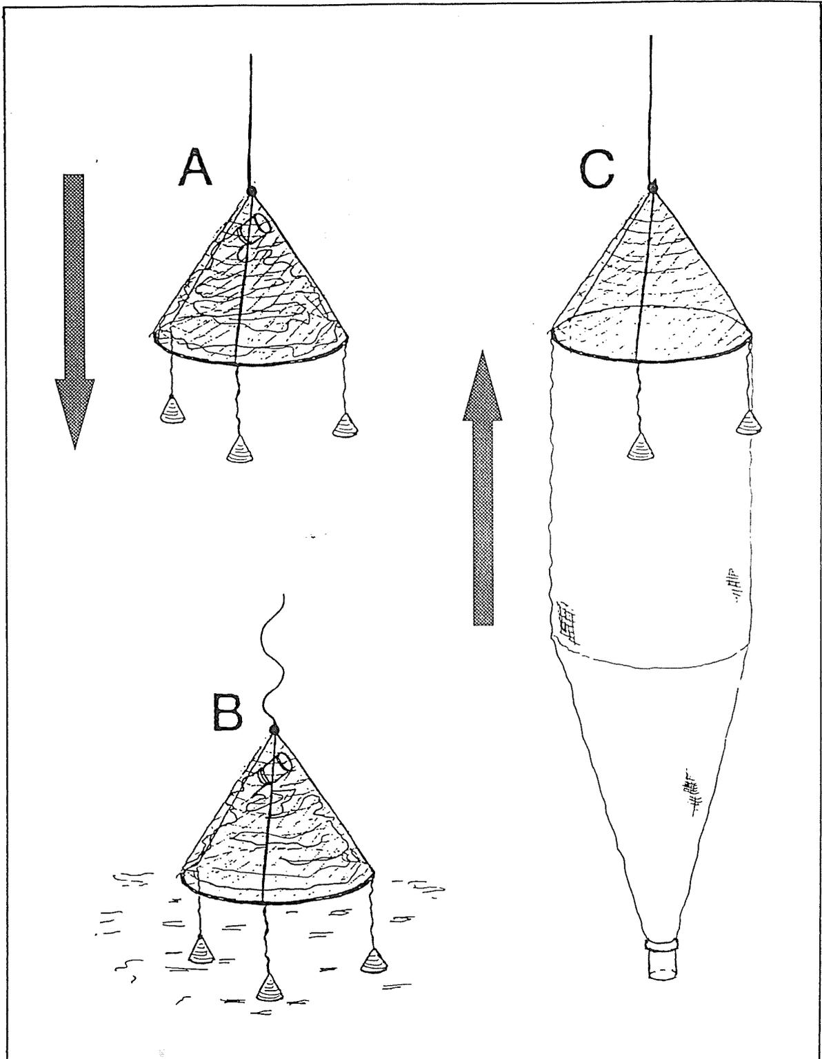
Figure 2.2 The vertical haul plankton net (A) in the lowering configuration; (B) in the the bottom resting configuration; and (C) in vertical haul configuration.
