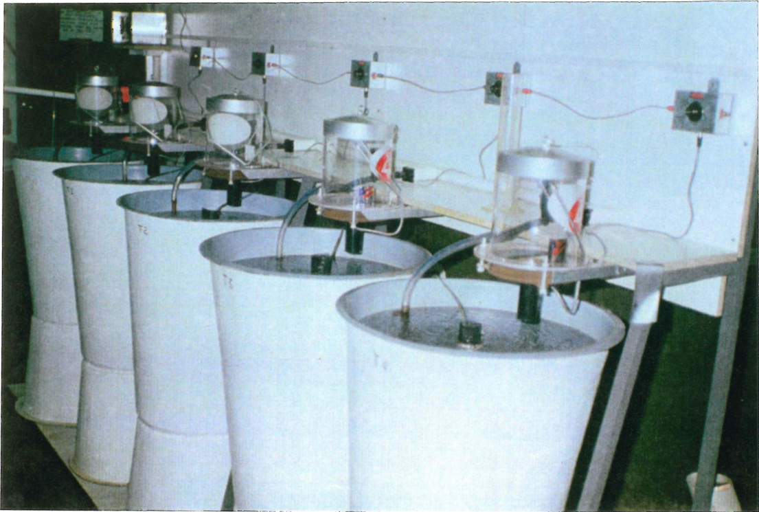
Figure 6.1. The experimental set-up, showing the conical rearing containers, automatic feed dispensers and electronic control boxes for each dispenser.
