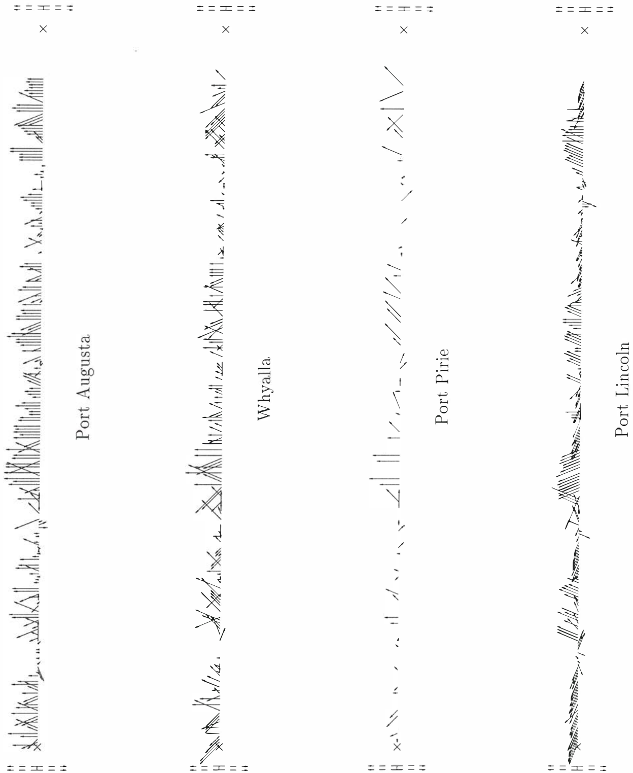
Figure vi.4: Vector time-series of winds measured by the BOM at surface wind stations Port Augusta, Whyalla, Port Pirie, and Port Lincoln during February 1988. The scale vectors at left and right represent wind speeds of 10 \text{ m s}^{-1} at a time interval of 4 h directed towards the north (up) and the south (down). The crosses at left and right represent 00:00 hrs on the first of the month and 00:00 hrs 31 d later, respectively. Winds of zero amplitude have no directional arrows and thus appear as dots.
