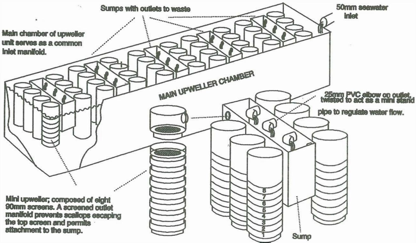
Fig 5.4.1 Experimental upweller unit
