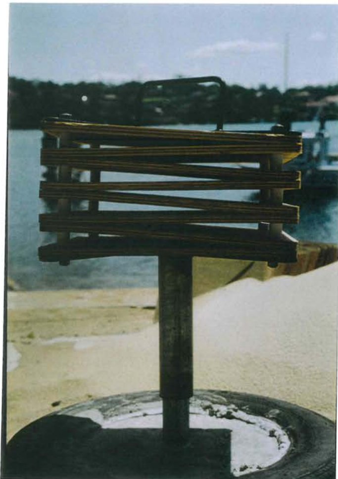
Figure 2.1(b) Crevice-type collector designed by Booth and Tarring (1986).
