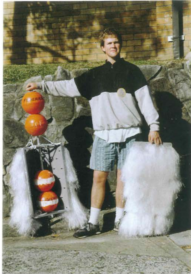
Figure 2.1(a) Seaweed-type collector designed by Phillips (1972).
