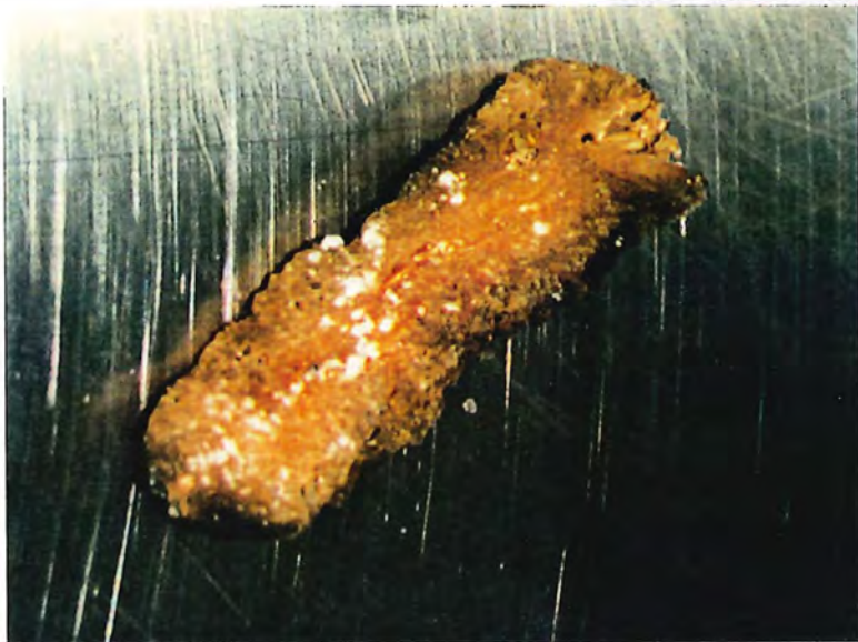
Plate No. 8: An Example Of Severe Pitting And Surface Breakdown Due To Excessive Exposure To Bromelain Activity
