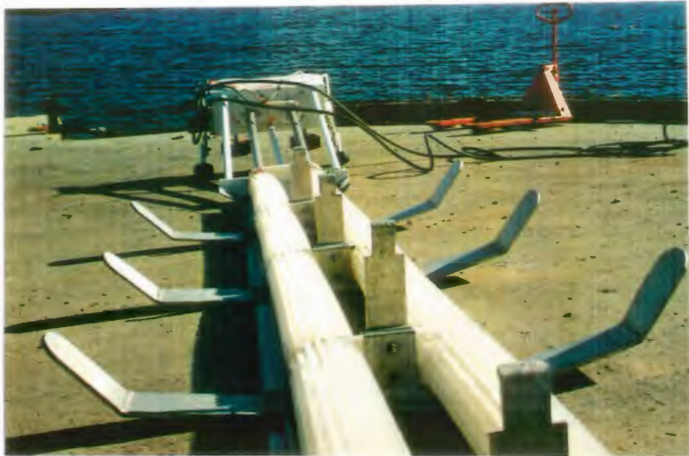
Figure 3. Prototype net cleaner showing lateral, aluminium side arms, designed to help stop twisting of brush lines
