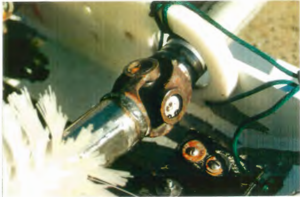
Figure 8. Aluminium spacer designed to reduce the contact angle between the top brushes and nets on some pens
