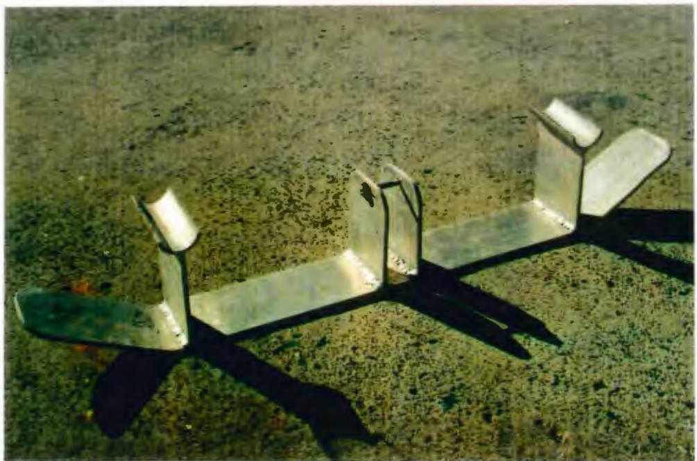
Figure 8. Aluminium spacer designed to reduce the contact angle between the top brushes and nets on some pens
