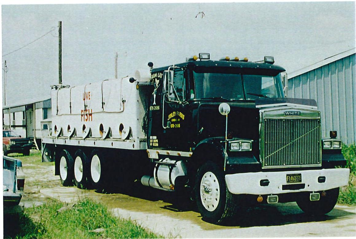
**Figure 2** Large live fish transport trucks used to transport fish to interstate markets in the continental US and in Canada.
