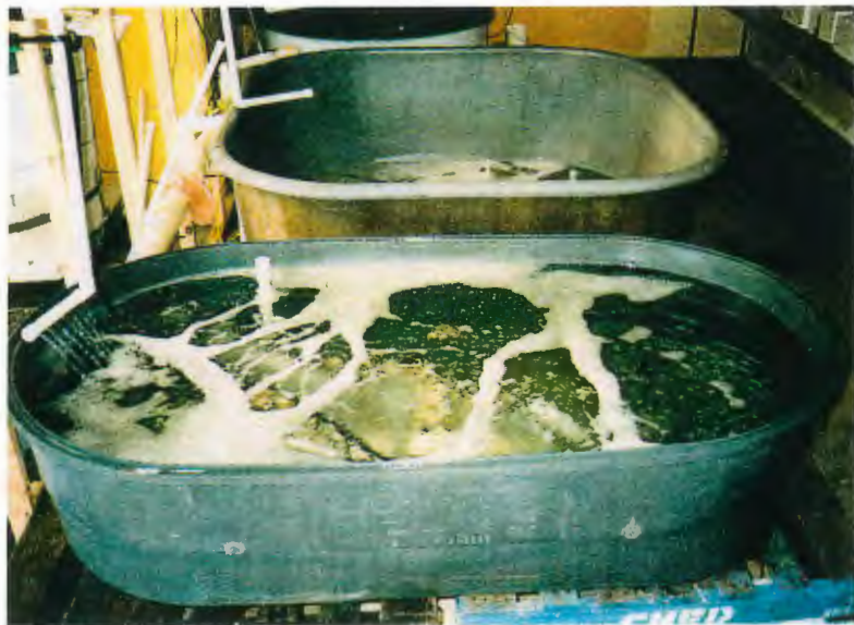
Figure 18 Different tank designs used in fish holding facilities. In the foreground, a shallow 'Rein' tank ideal for fishes that require little depth, such as flatfishes. Behind, a 'Rathburn' type tank, which is ideal for general use.
