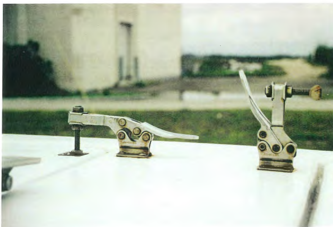
Figure 6 (Above) lid of live fish transport tank, showing vent for gas exchange and locking prop. (Below) 'De-Sta-Co' latches in latched (left) and unlatched (right) positions.
