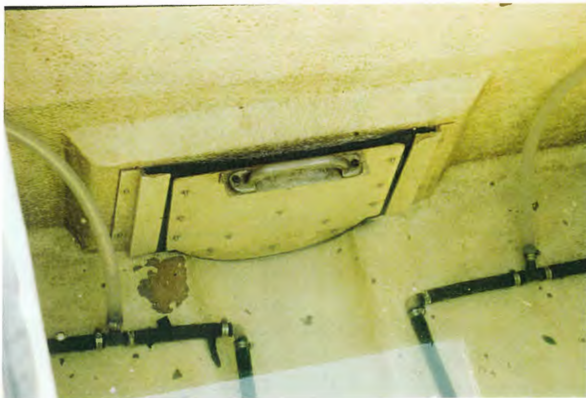
Figure 7 Inside view of live fish transport tank showing gate valve, drain trough, and oxygen diffusers constructed from rubber soaker hose.
