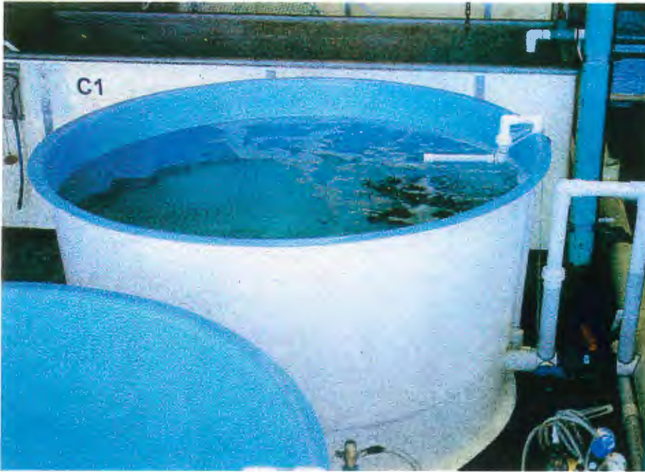
Figure 19 Circular fibreglass tank used for holding barramundi. Note the external standpipe which regulates the water level, the outlet valve used to completely drain the tank, and the horizontal spray bar which promotes circular water movement within the tank.
