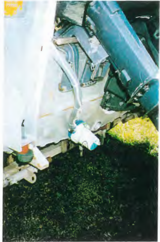
Figure 2 Stern view of catching dinghy showing 12-volt pump for water supply to live fish well. The use of pumps to supply water to live wells provides better water quality and reduces fish mortality.
