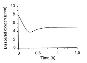
Figure 12 Dissolved oxygen concentration in transport tank after loading fish (Johnson 1979).
