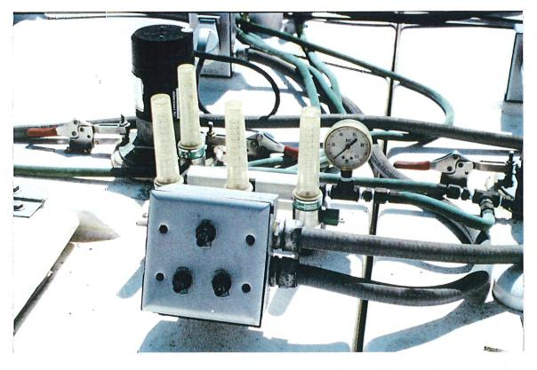
Figure 15 (Above) Cab of live fish transport truck showing display unit for dissolved oxygen sensors fitted to tanks, and low oxygen pressure alarm. (Below) Live fish transport tanks showing oxygen supply system and individual flow controls for each diffuser, agitators (3 per tank) and switches.
