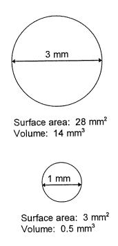
Figure 11 Surface area and volume for 1 and 3 mm diameter oxygen bubbles.
