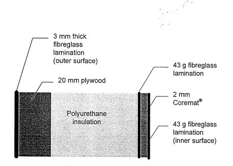
**Figure 5** Details of wall construction of live fish transport tanks made by Peterson Fibreglass Laminates Inc., Shell Lake, Wisconsin, USA. (Not to scale).
