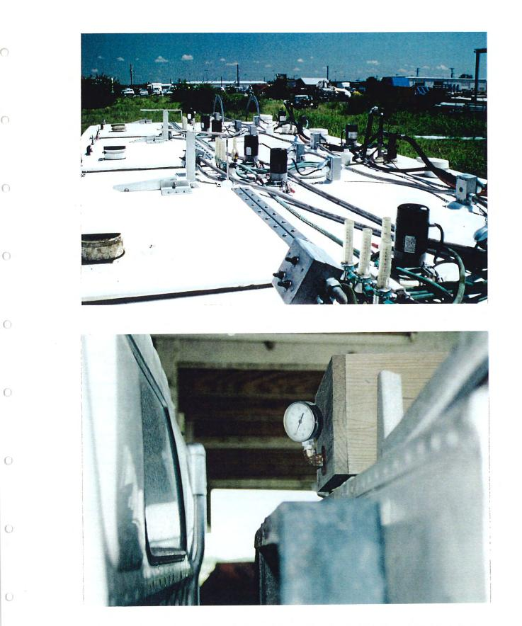
**Figure 14** (Above) Controls for live fish transport tank, including: individual flow controls for each air diffuser, oxygen supply system pressure gauge, individual switches for agitators. Note agitator held in place with 'De-Sta-Co' latches, plugged into waterproof 12V power supply. (Below) Oxygen supply system pressure gauge, located to be visible in driver's rear view mirror.
