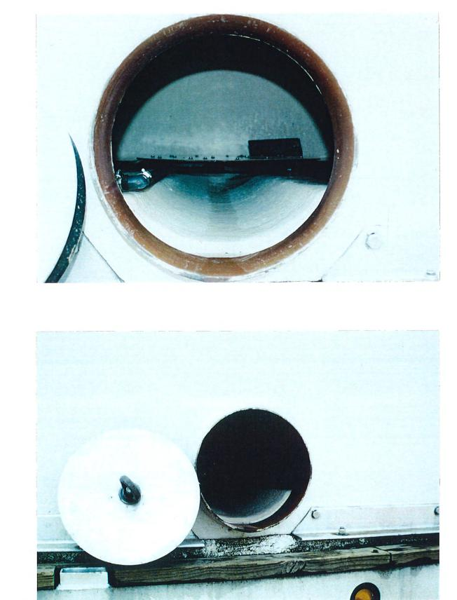
**Figure 8** (Above) View inside live fish transport tank, with gate valve removed, from drain. (Below) External view of tank drain with external plug removed.
