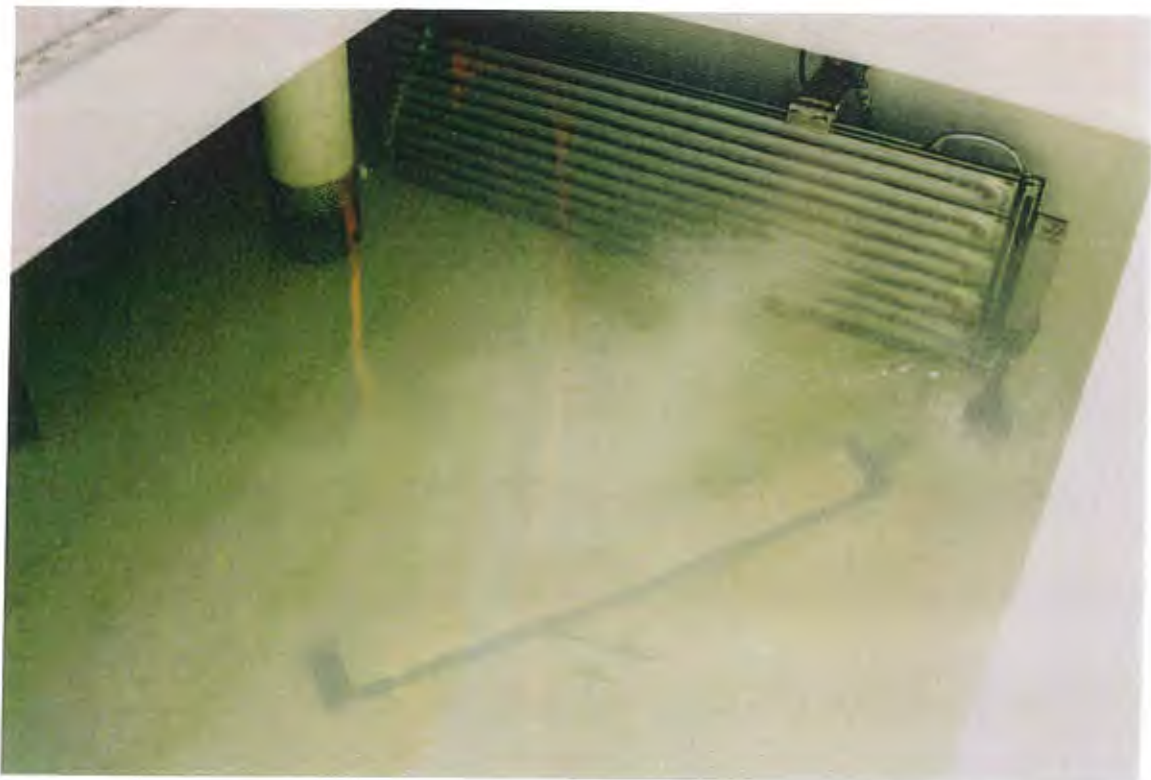
Figure 9 (Above) Refrigerative cooling system fitted to live fish transport truck. (Below) Cooling coils of refrigerative system in live fish transport tank. Note cloud of fine bubbles from oxygen diffuser. White tube at left is an agitator, with black plastic mesh screen fitted to protect small fish from agitator turbulence.
