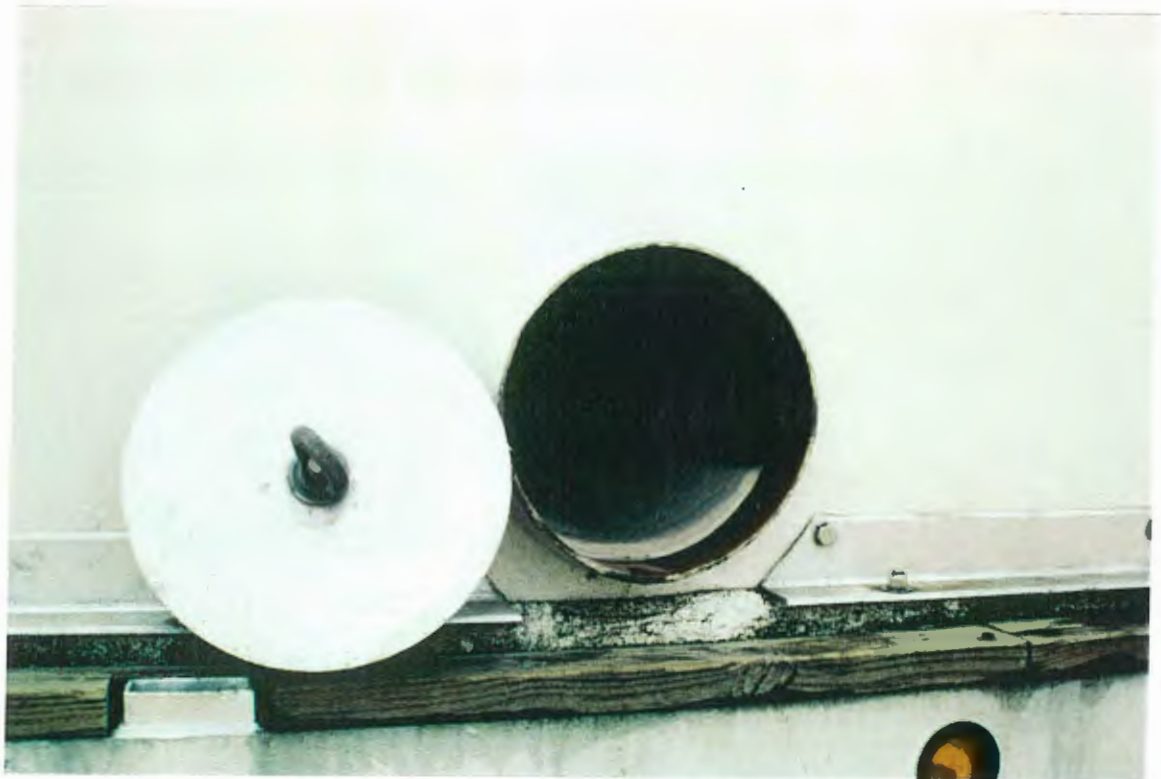
Figure 8 (Above) View inside live fish transport tank, with gate valve removed, from drain. (Below) External view of tank drain with external plug removed.
