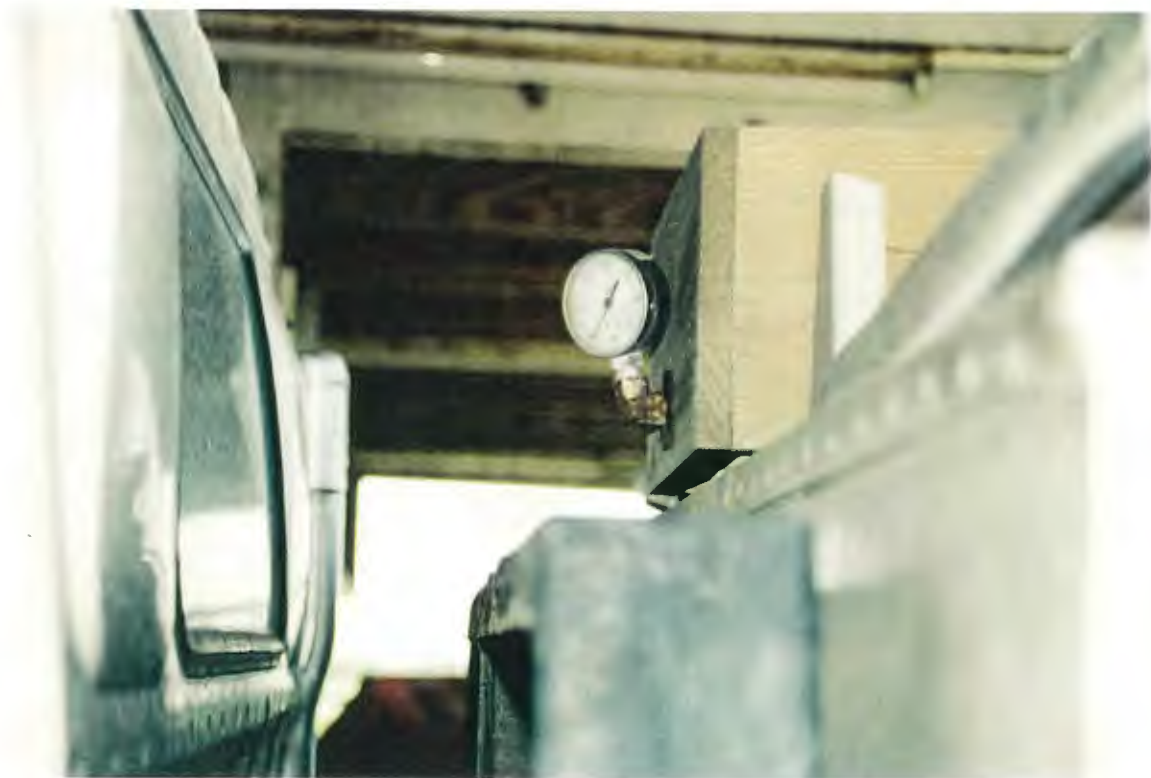
Figure 14 (Above) Controls for live fish transport tank, including: individual flow controls for each air diffuser, oxygen supply system pressure gauge, individual switches for agitators. Note agitator held in place with 'De-Sta-Co' latches, plugged into waterproof 12V power supply. (Below) Oxygen supply system pressure gauge, located to be visible in driver's rear view mirror.
