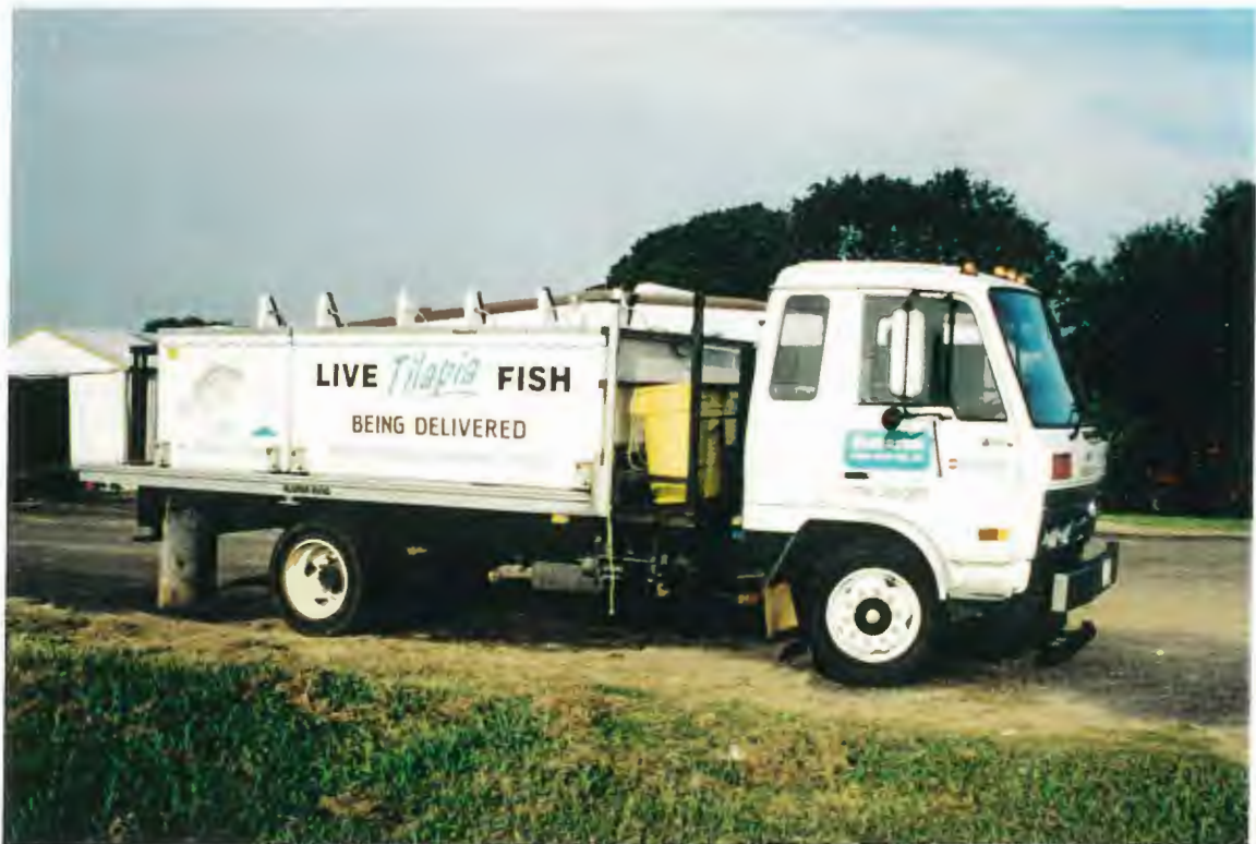
Figure 1 Smaller live fish transport trucks used to carry fish to local markets.
