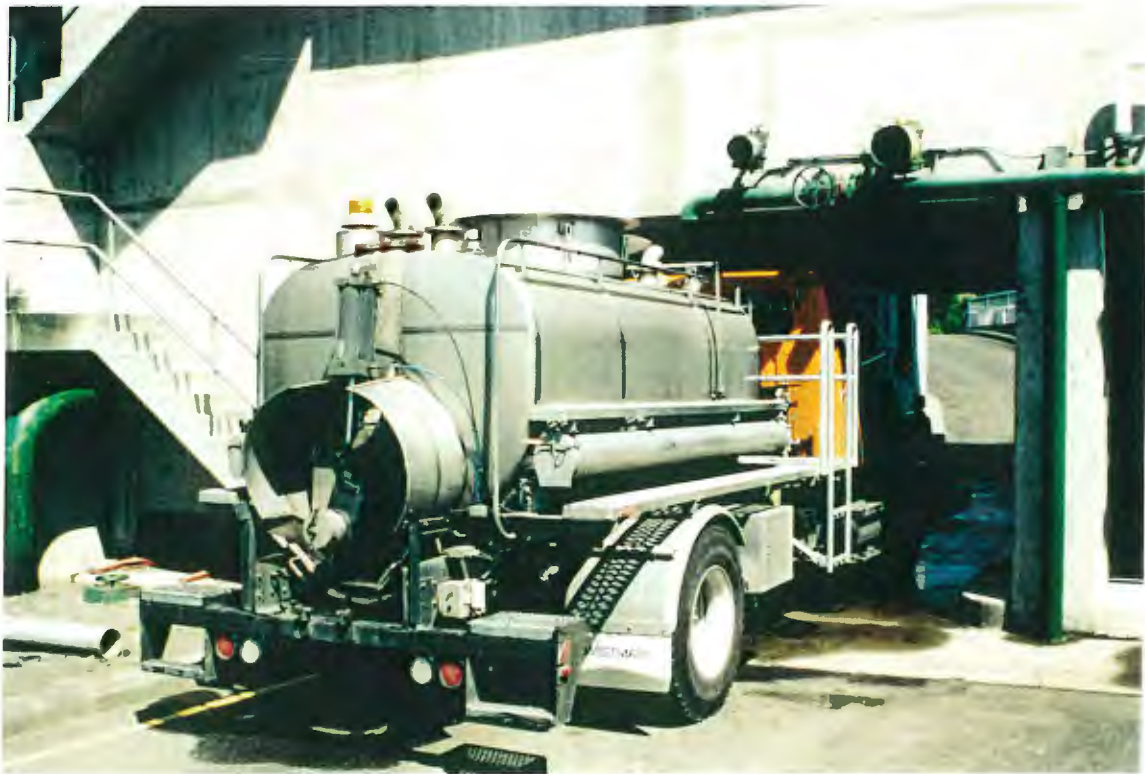
Figure 16 Handling free loading system in use at Kalama State Fish Hatchery, Washington. Fish are loaded from an overhead tank via a flexible coupling (above) that connects to a hatch on the top of the transport tank (below). When the valves on the truck tank are opened, the water and fish in the overhead tank drain into the truck tank.
