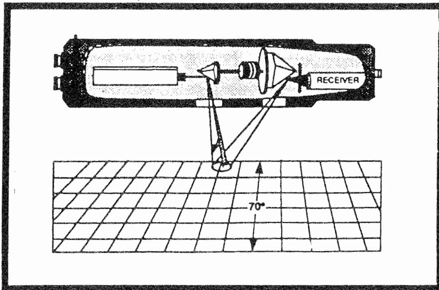
Synchronized Detector Optics Track a Single Point of Illumination, Minimizing the Effect of Backscatter in the Water Column
