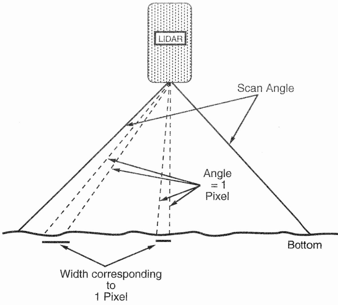
Geometry of path scanning by towed body LIDAR, comparing a fixed (= 1 pixel) angle immediately below the tow path with the same 1-pixel angle to one side of the tow path, showing effect on area of the bottom integrated into the single pixel datum.
