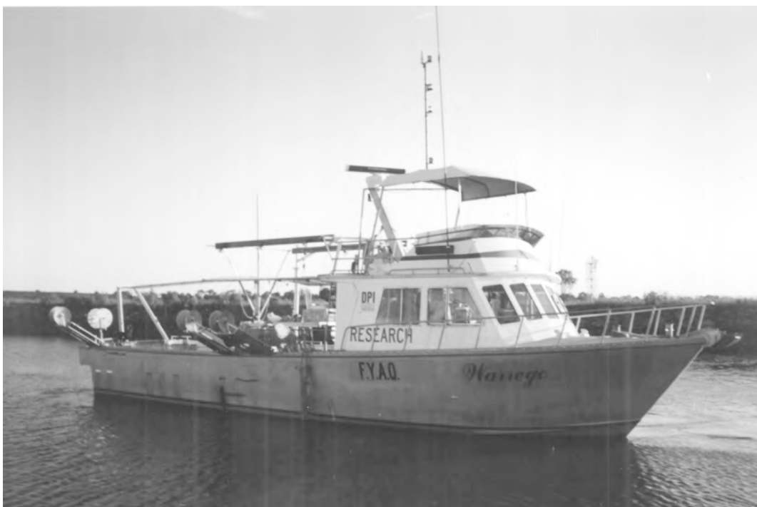
Figure 3. Jigging machines and hand spools with outriggers mounted on QDPI's research vessel, Warrego.
