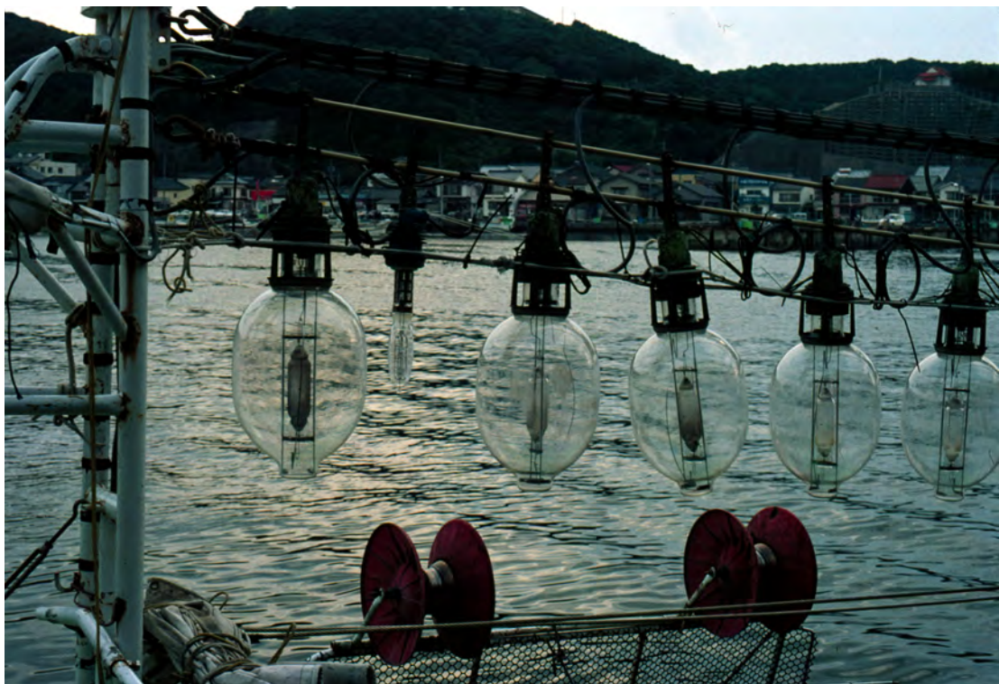
Figure B12. Fluorescent and halogen bulbs (3-5 kW).
