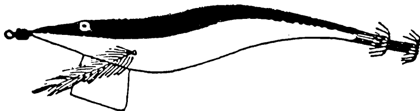
Figure 6. Typical design of a prawn-shaped trolling jig, lead weight under the head and a double row of barbless hooks trailing (the upper colour is either red or green with dark stripes) - after Hamabe et al., 1982.
