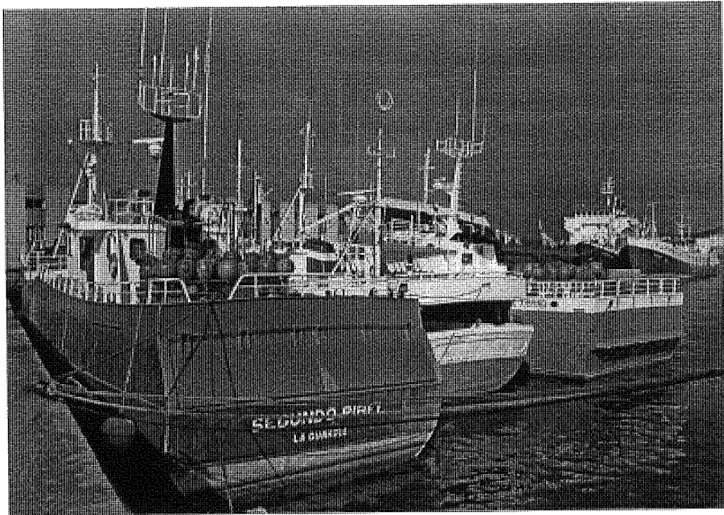
Figure 13b. A more modern longline vessel showing closed hatch covers. Note however, in both vessels the crew work in a fully enclosed area.
