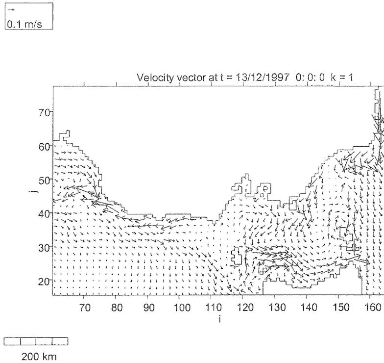
**Figure 9C.** Surface (0-5 m) current vectors predicted by hydrodynamic modelling for southeastern Australia during Cruise 2 at 00:00 h on December 13, 1997. Arrows indicate current direction; length of lines are proportional to current velocity (m/s).
