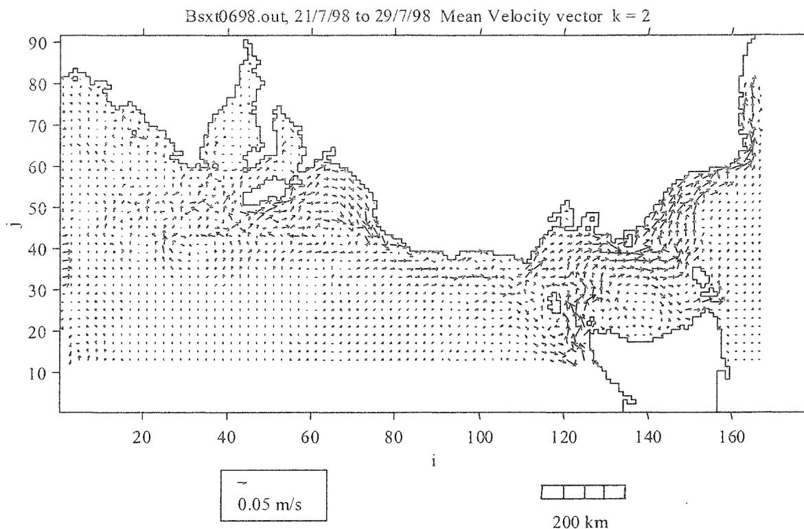
**Figure 8B.** Simulated hydrodynamic current model of southeastern Australia at a depth of 5-15 m obtained for the period 21-29 July 1998 (Cruise 4). Arrows indicate current direction; length of lines are proportional to current velocity (m/s).
