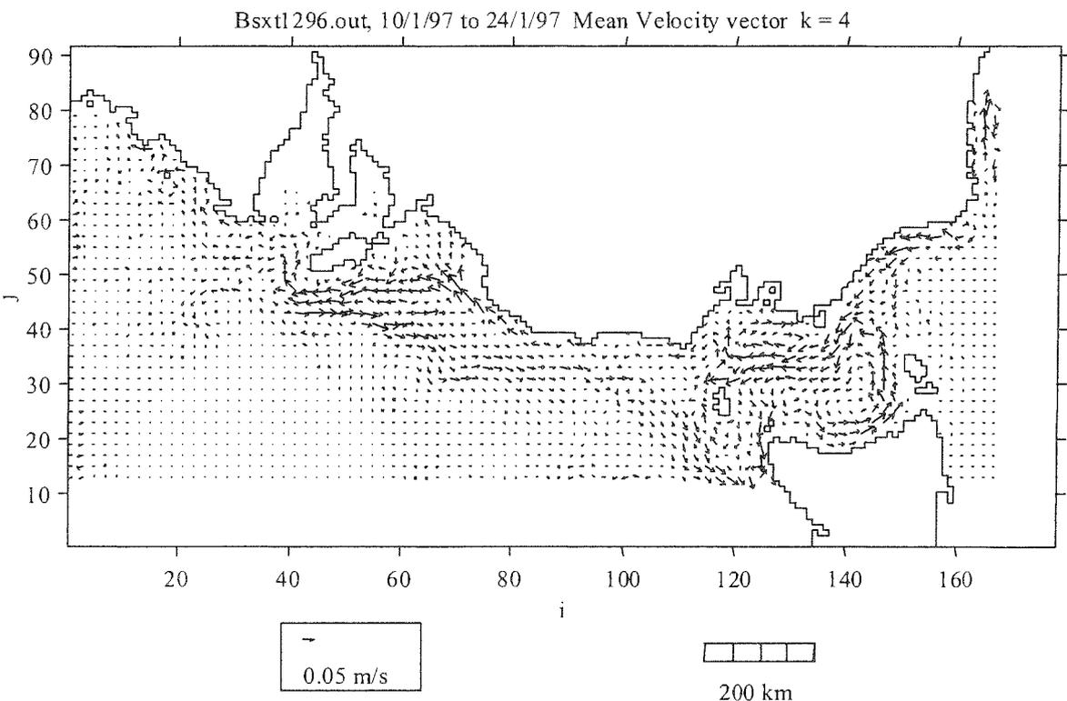
**Figure 5D.** Simulated hydrodynamic current model of southeastern Australia at a depth of 35-55 m obtained for the period 10-24 January 1997 (Cruise 1). Arrows indicate current direction; length of lines are proportional to current velocity (m/s).
