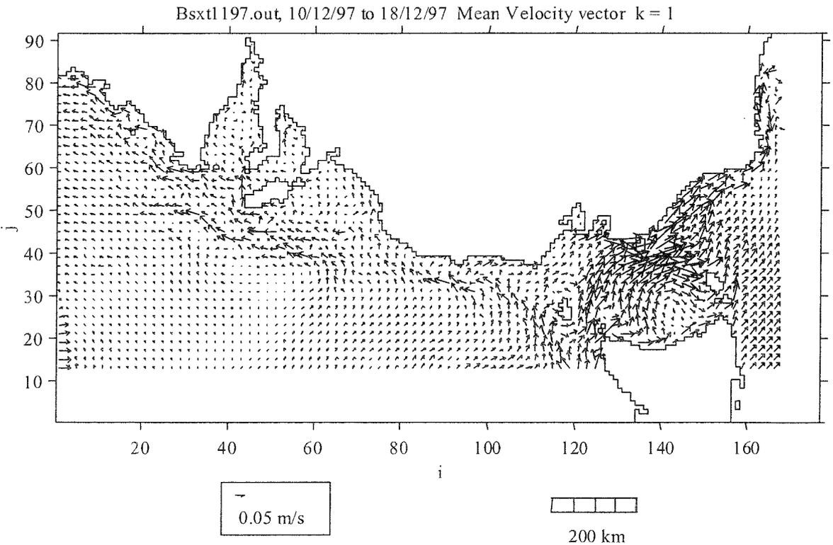
**Figure 6A.** Simulated hydrodynamic current model of southeastern Australia at a depth of 0-5 m obtained for the period 10-18 December 1997 (Cruise 2). Arrows indicate current direction; length of lines are proportional to current velocity (m/s).
