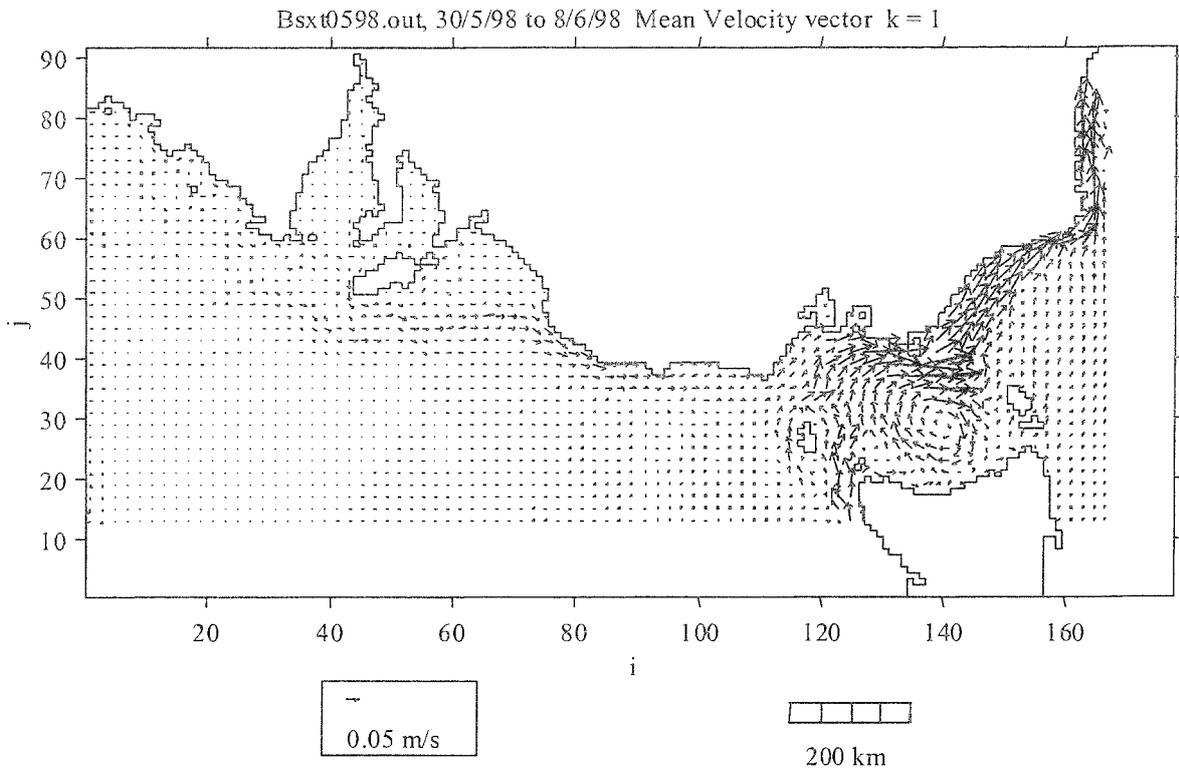
**Figure 7A.** Simulated hydrodynamic current model of southeastern Australia at a depth of 0-5 m obtained for the period 30 May to 8 June 1998 (Cruise 3). Arrows indicate current direction; length of lines are proportional to current velocity (m/s).
