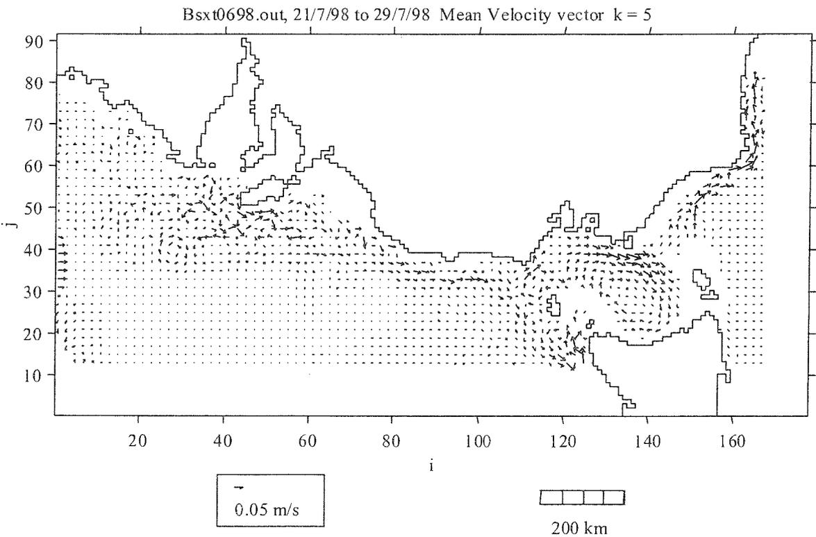
**Figure 8E.** Simulated hydrodynamic current model of southeastern Australia at a depth of 55-75 m obtained for the period 21-29 July 1998 (Cruise 4). Arrows indicate current direction; length of lines are proportional to current velocity (m/s).
