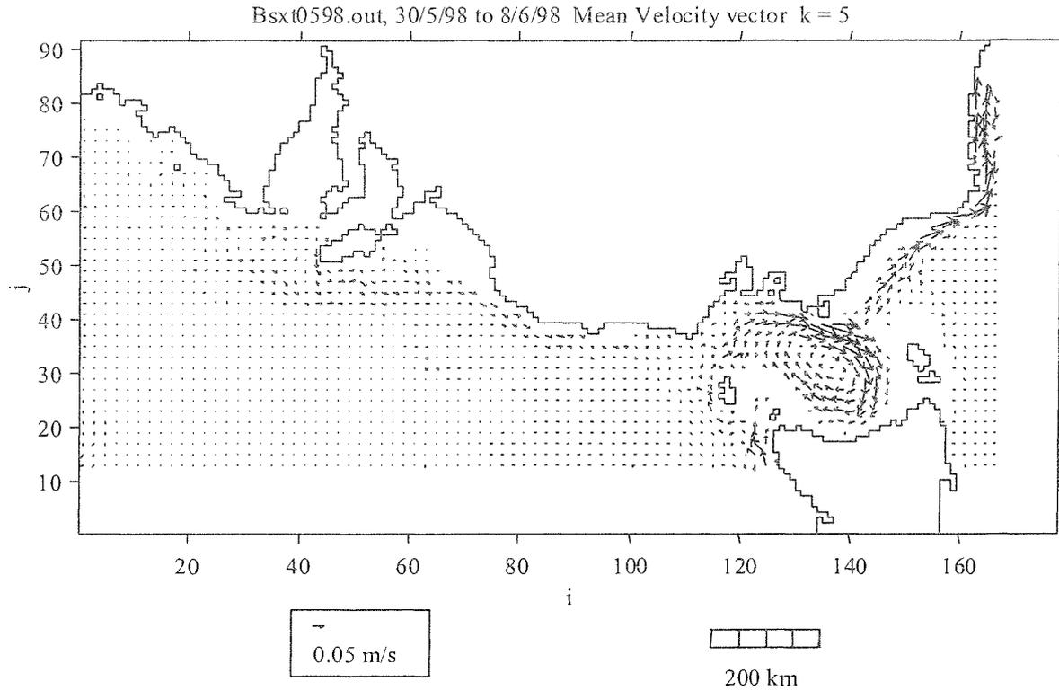
**Figure 7E.** Simulated hydrodynamic current model of southeastern Australia at a depth of 55-75 m obtained for the period 30 May to 8 June 1998 (Cruise 3). Arrows indicate current direction; length of lines are proportional to current velocity (m/s).
