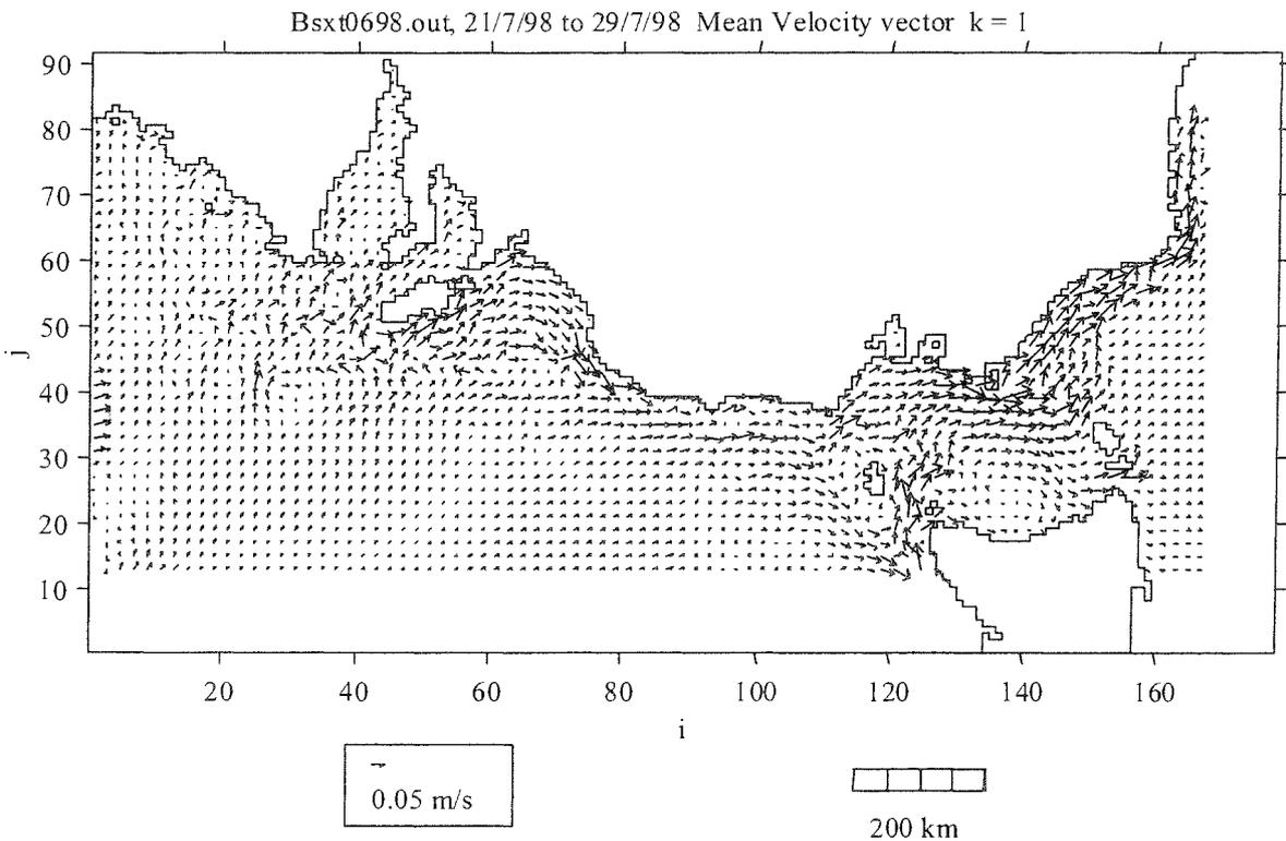
**Figure 8A.** Simulated hydrodynamic current model of southeastern Australia at a depth of 0-5 m obtained for the period 21-29 July 1998 (Cruise 4). Arrows indicate current direction; length of lines are proportional to current velocity (m/s).
