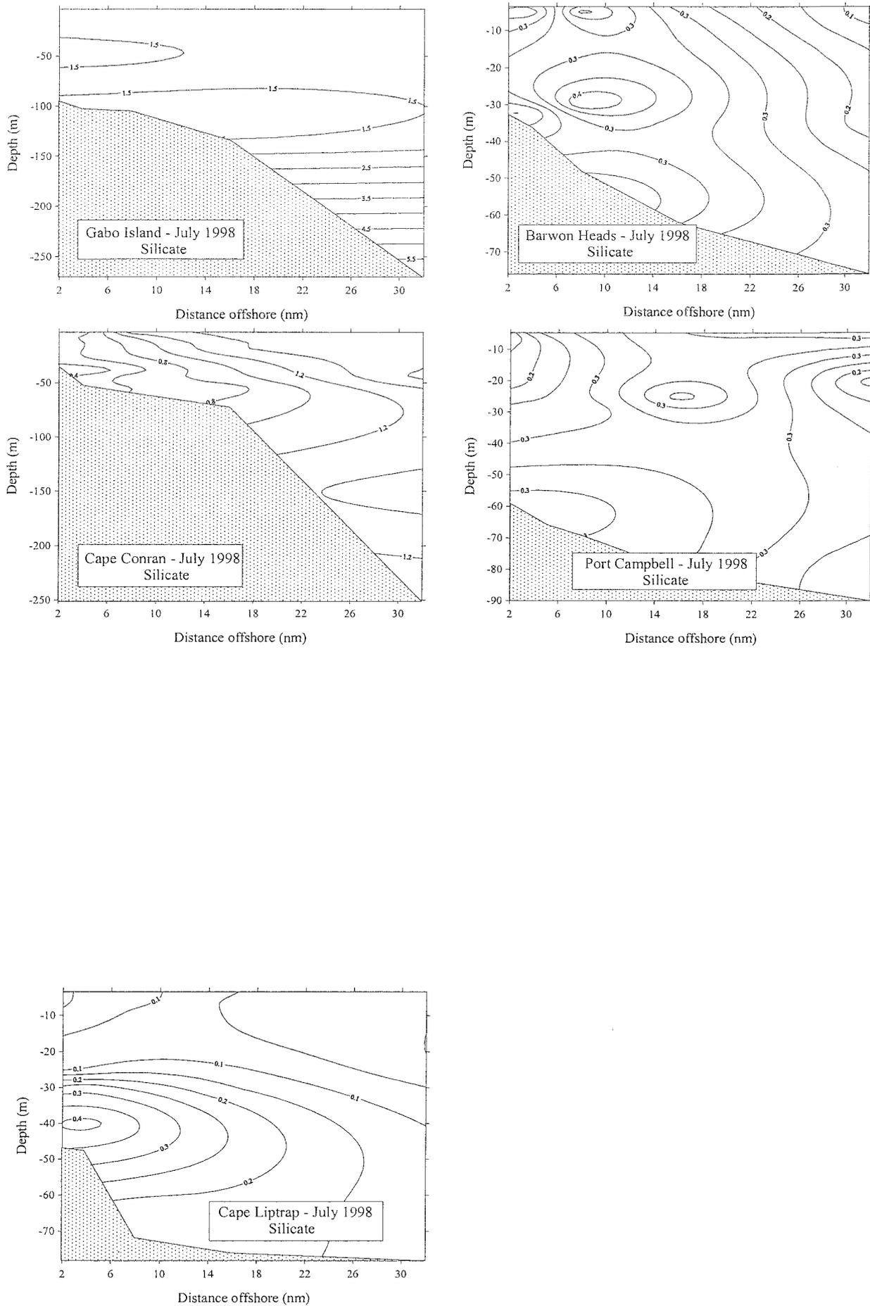
Figure 17D. Vertical silicate profiles in transects 1 (Gabo Island) to 6 (Port Campbell) in southeastern Australia during cruise 4 (Jul 1998). Transect 3 (Seaspray) was not sampled; data for transects 7 (Portland) and 8 (Port MacDonnell) are incomplete.
