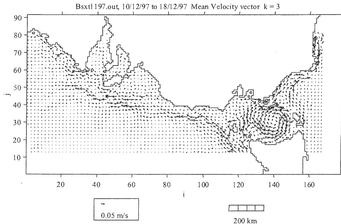
**Figure 6C.** Simulated hydrodynamic current model of southeastern Australia at a depth of 15-35 m obtained for the period 10-18 December 1997 (Cruise 2). Arrows indicate current direction; length of lines are proportional to current velocity (m/s).
