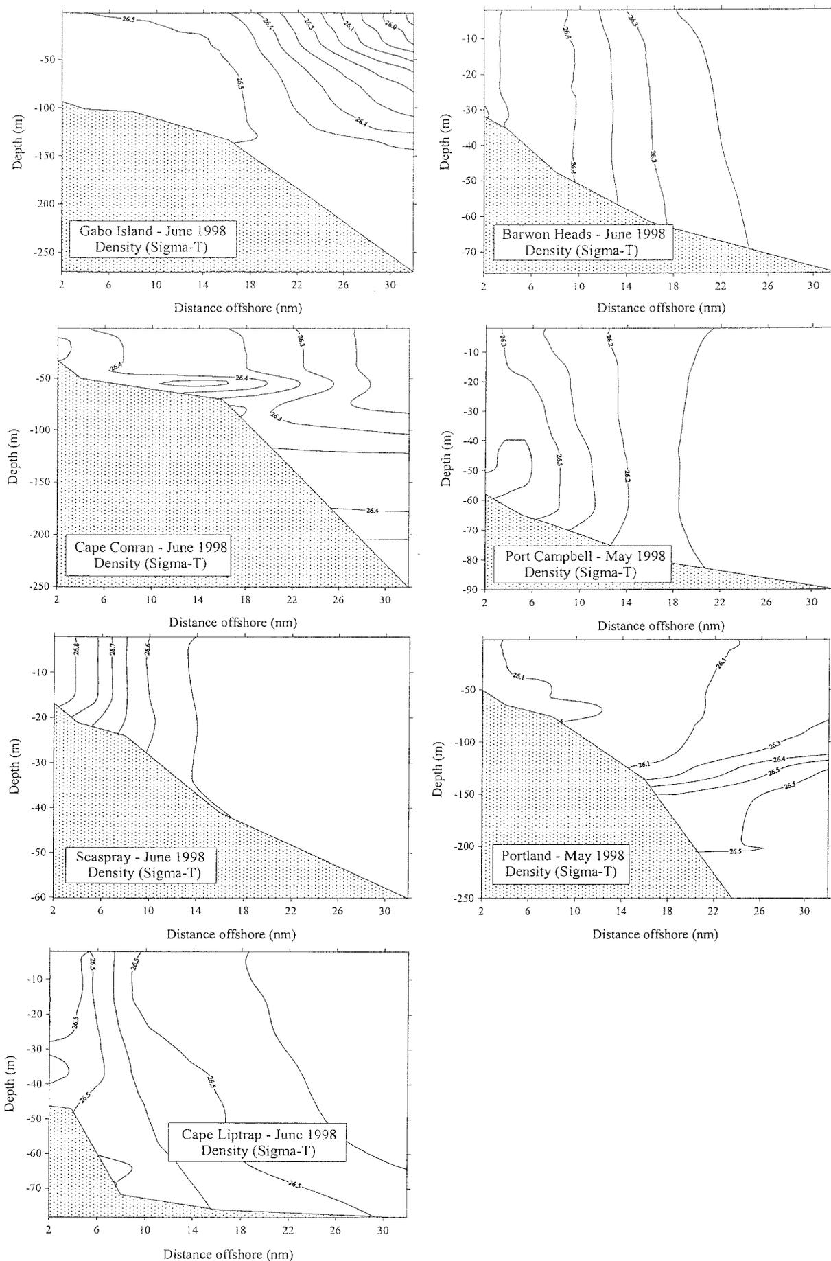
Figure 14C. Vertical density profiles (Sigma-T) in transects 1 (Gabo Island) to 7 (Portland) in southeastern Australia during cruise 3 (May-Jun 1997). Transect 8 (Port MacDonnell) was not sampled.
