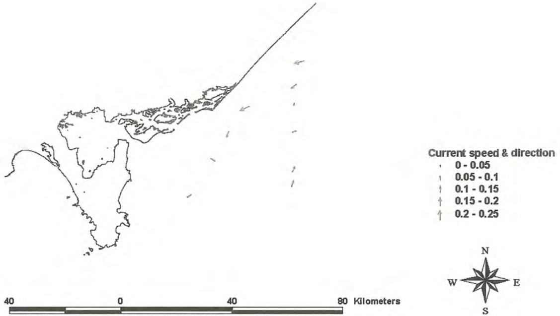
**Figure 10.** Tidally corrected shipboard ADCP current measurements for the area just east of Wilsons Promontory during cruise 2 on the 12/13 of December, 1997. Arrows indicate current direction; length of lines are proportional to current velocity (m/s).
