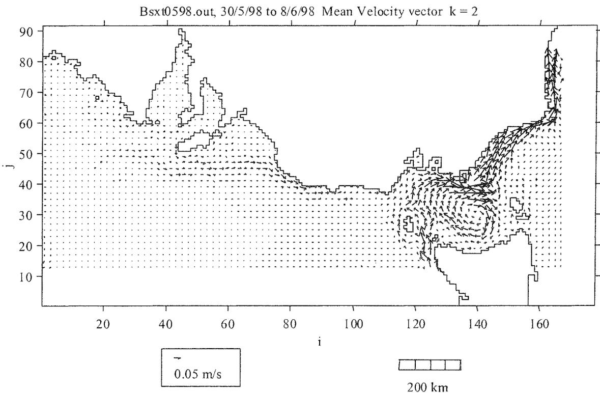
**Figure 7B.** Simulated hydrodynamic current model of southeastern Australia at a depth of 5-15 m obtained for the period 30 May to 8 June 1998 (Cruise 3). Arrows indicate current direction; length of lines are proportional to current velocity (m/s).
