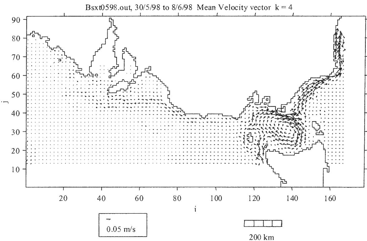
**Figure 7D.** Simulated hydrodynamic current model of southeastern Australia at a depth of 35-55 m obtained for the period 30 May to 8 June 1998 (Cruise 3). Arrows indicate current direction; length of lines are proportional to current velocity (m/s).
