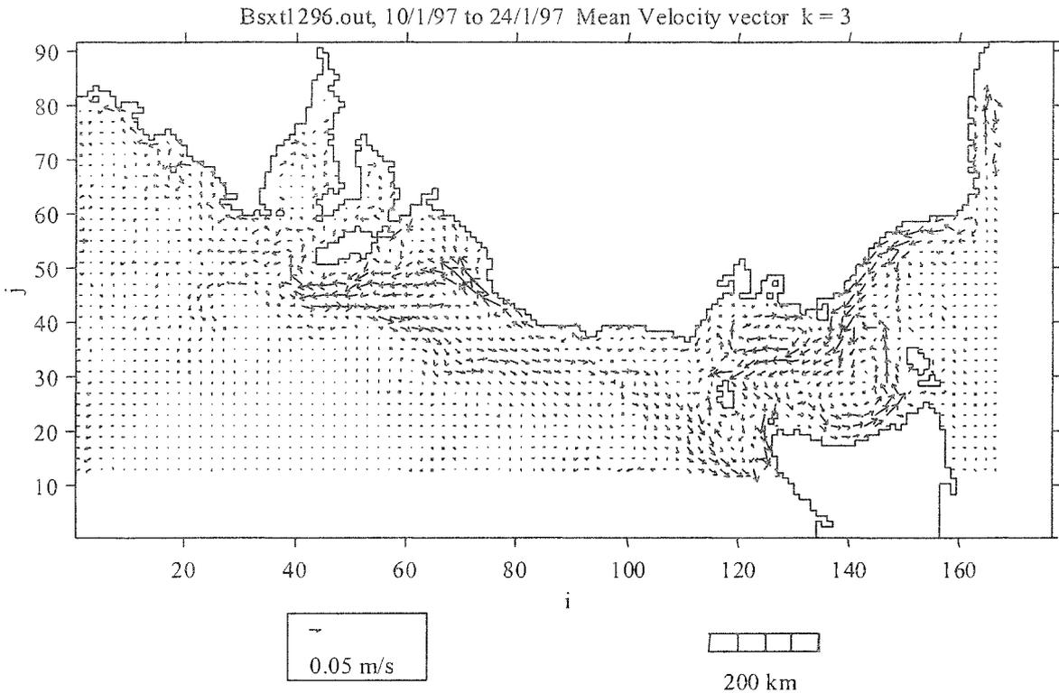
**Figure 5C.** Simulated hydrodynamic current model of southeastern Australia at a depth of 15-35 m obtained for the period 10-24 January 1997 (Cruise 1). Arrows indicate current direction; length of lines are proportional to current velocity (m/s).
