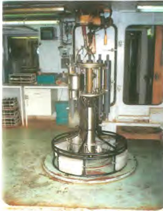
**Figure 4.** The CSIRO CTD rosette used in this study showing five Niskin bottles.
