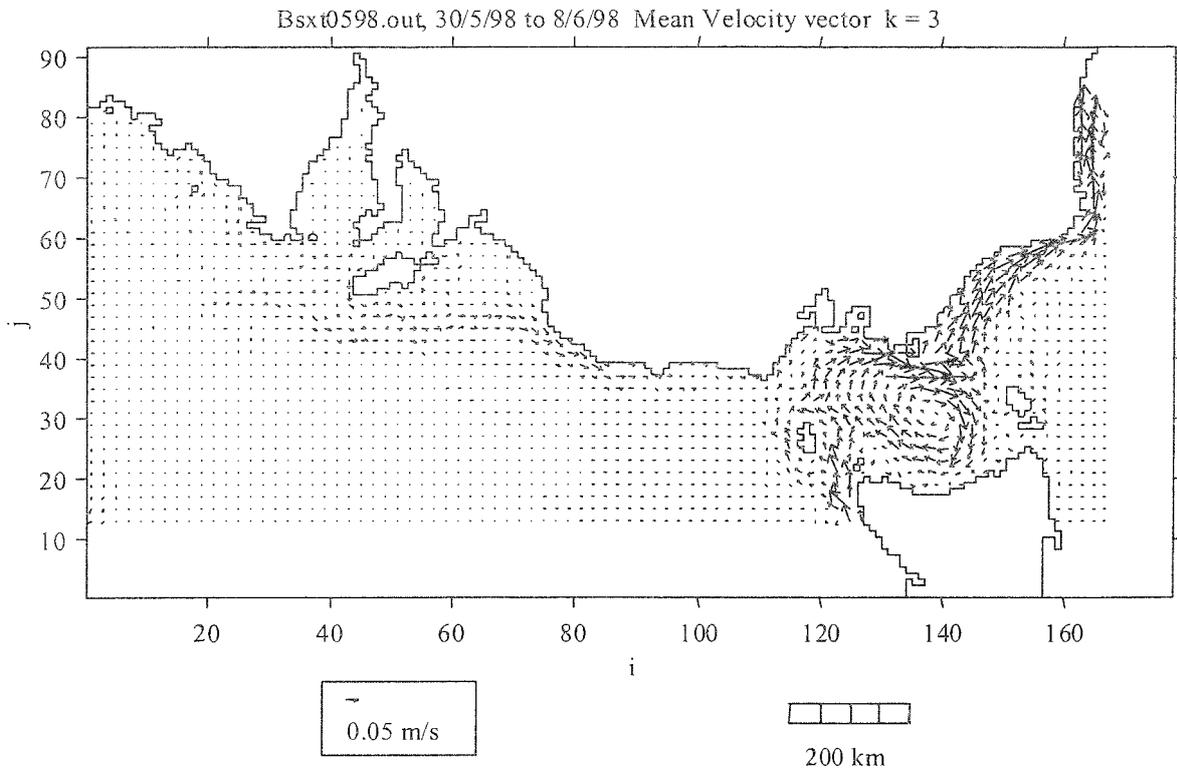
**Figure 7C.** Simulated hydrodynamic current model of southeastern Australia at a depth of 15-35 m obtained for the period 30 May to 8 June 1998 (Cruise 3). Arrows indicate current direction; length of lines are proportional to current velocity (m/s).
