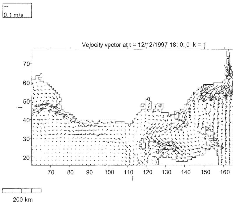
**Figure 9B.** Surface (0-5 m) current vectors predicted by hydrodynamic modelling for southeastern Australia during Cruise 2 at 18:00 h on December 12, 1997. Arrows indicate current direction; length of lines are proportional to current velocity (m/s).
