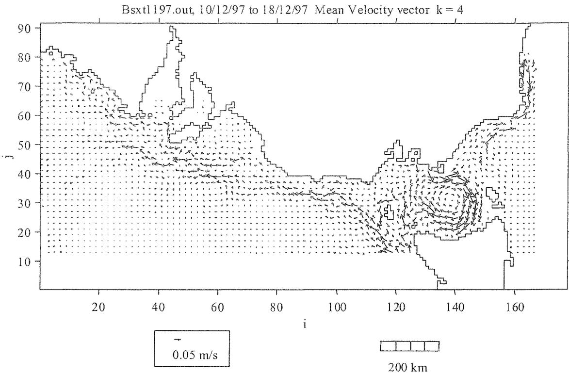
**Figure 6D.** Simulated hydrodynamic current model of southeastern Australia at a depth of 35-55 m obtained for the period 10-18 December 1997 (Cruise 2). Arrows indicate current direction; length of lines are proportional to current velocity (m/s).
