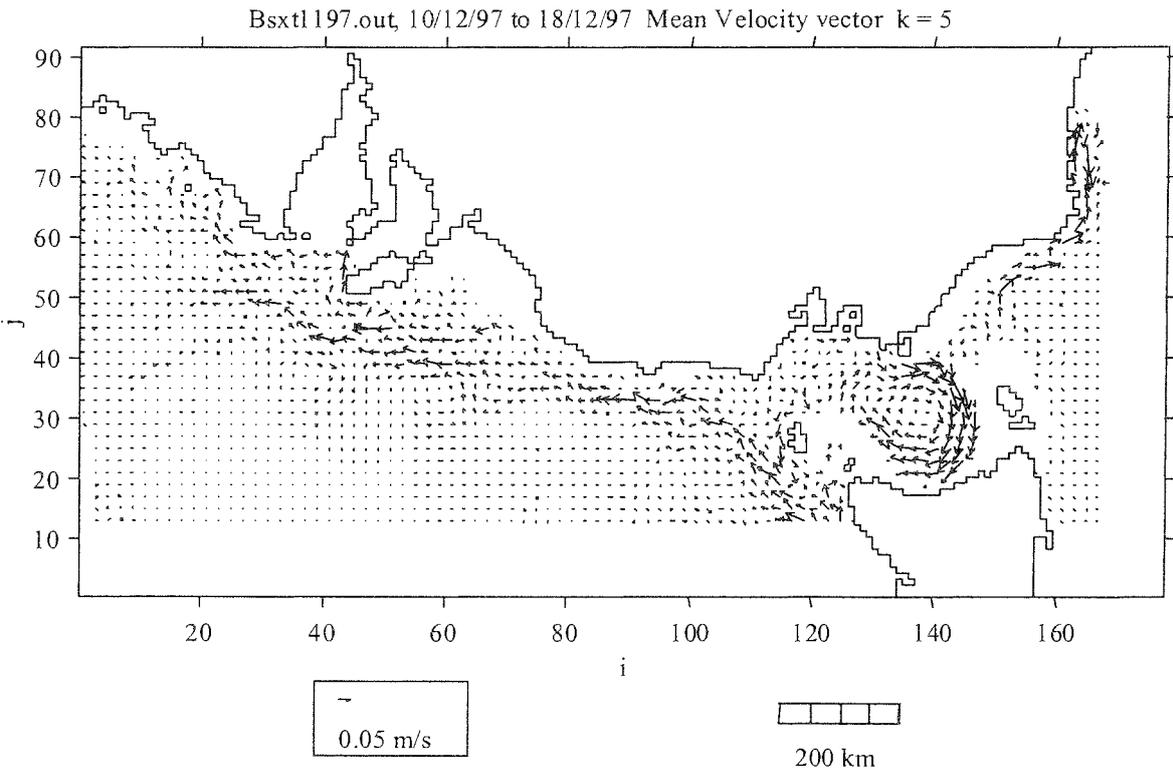
**Figure 6E.** Simulated hydrodynamic current model of southeastern Australia at a depth of 55-75 m obtained for the period 10-18 December 1997 (Cruise 2). Arrows indicate current direction; length of lines are proportional to current velocity (m/s).
