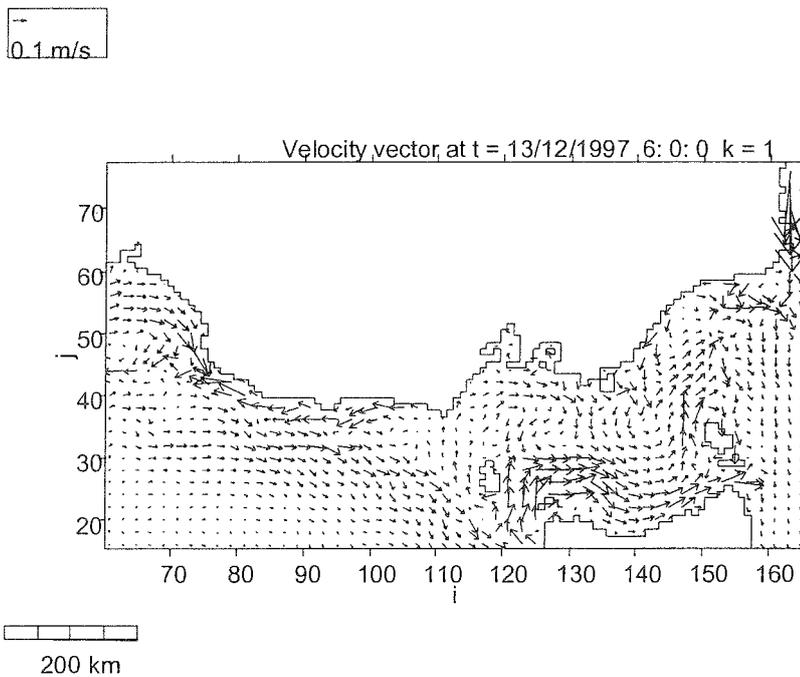
**Figure 9D.** Surface (0-5 m) current vectors predicted by hydrodynamic modelling for southeastern Australia during Cruise 2 at 06:00 h on December 13, 1997. Arrows indicate current direction; length of lines are proportional to current velocity (m/s).
