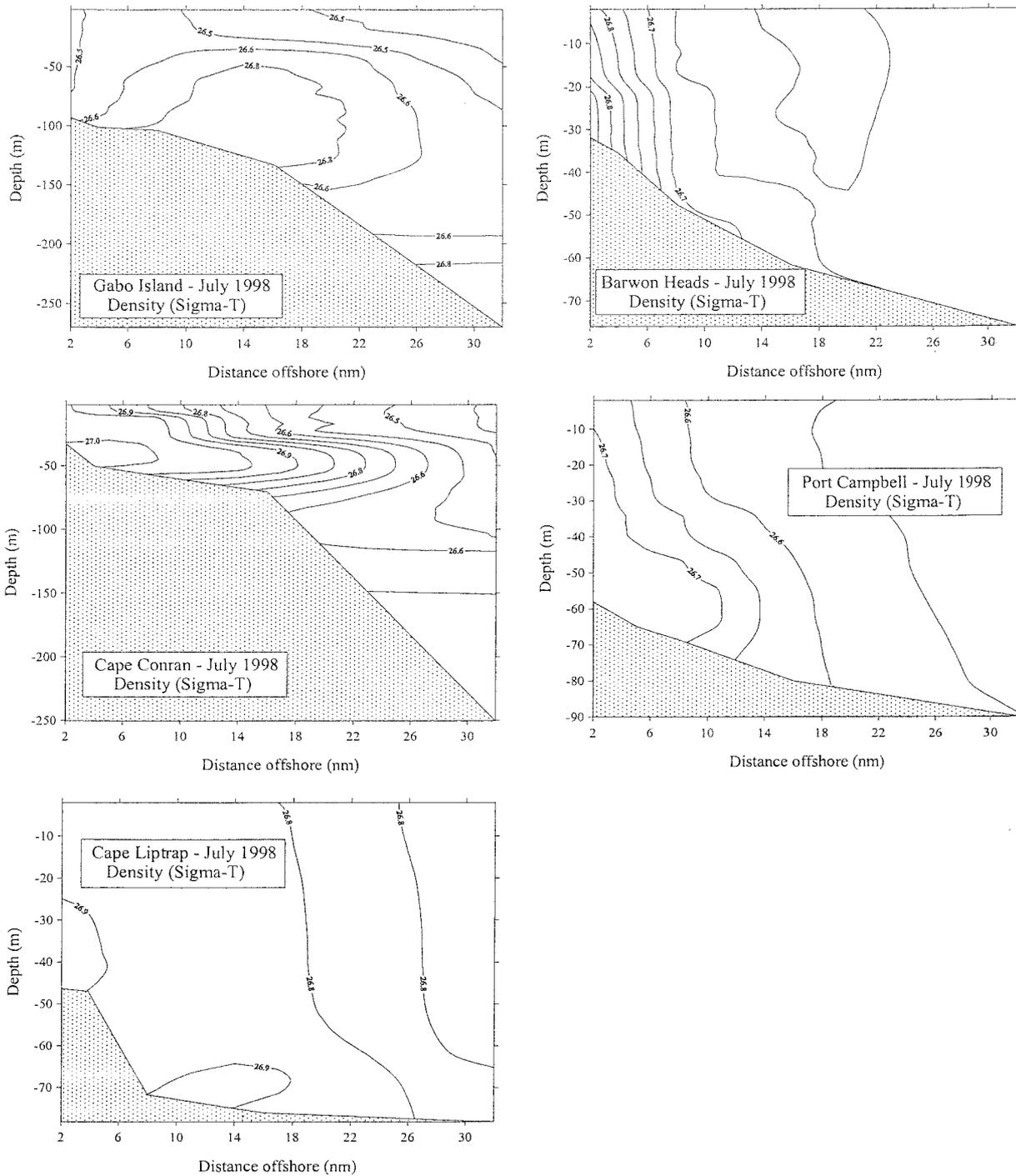
Figure 14D. Vertical density profiles (Sigma-T) in transects 1 (Gabo Island) to 6 (Port Campbell) in southeastern Australia during cruise 4 (Jul 1998). Transect 3 (Seaspray) was not sampled; data for transects 7 (Portland) and 8 (Port MacDonnell) are incomplete.
