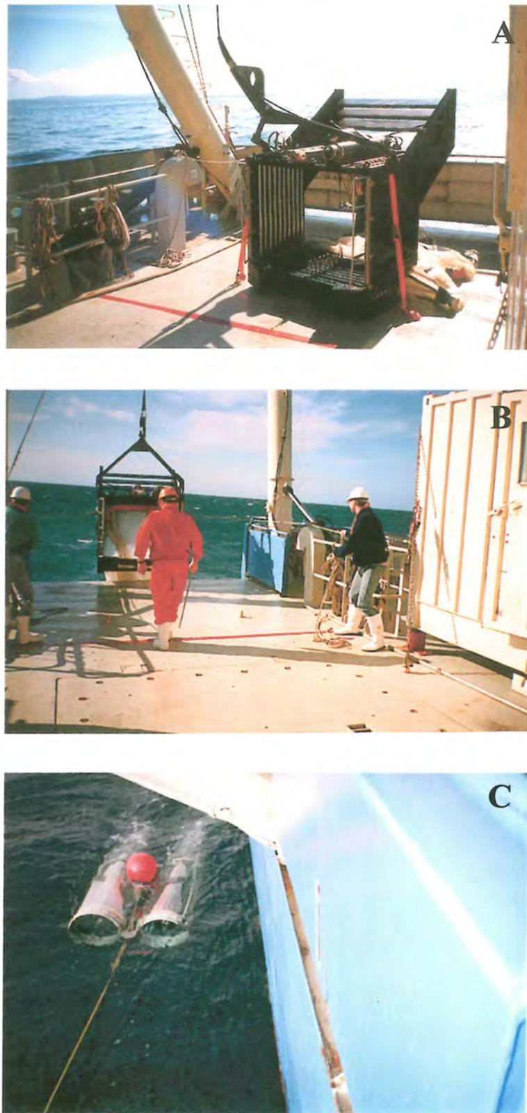
**Figure 3.** Plankton samplers employed during this study. (A, B) the CSIRO EZ net used for sampling plankton at different strata through the water column; (C) the MAFRI bongo sampler used for surface (neuston) and some of the 25-0 m tows.
