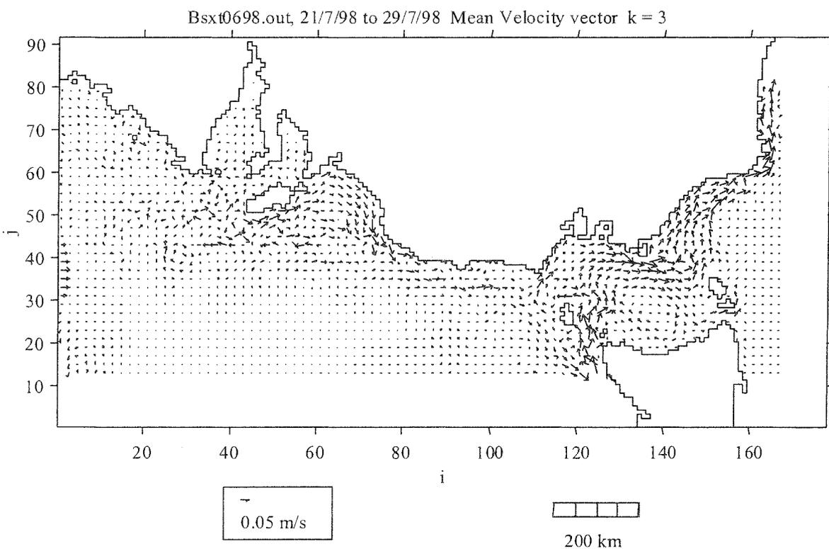
**Figure 8C.** Simulated hydrodynamic current model of southeastern Australia at a depth of 15-35 m obtained for the period 21-29 July 1998 (Cruise 4). Arrows indicate current direction; length of lines are proportional to current velocity (m/s).
