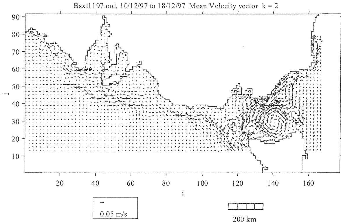
**Figure 6B.** Simulated hydrodynamic current model of southeastern Australia at a depth of 5-15 m obtained for the period 10-18 December 1997 (Cruise 2). Arrows indicate current direction; length of lines are proportional to current velocity (m/s).
