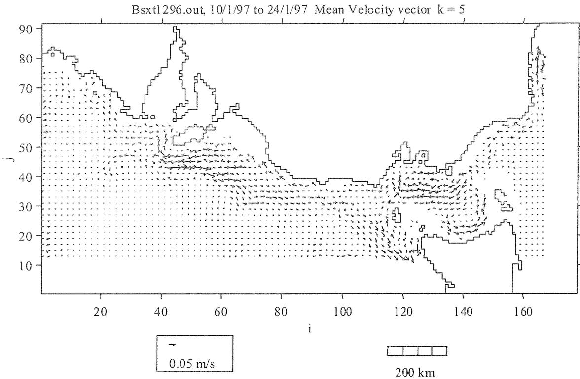
**Figure 5E.** Simulated hydrodynamic current model of southeastern Australia at a depth of 55-75 m obtained for the period 10-24 January 1997 (Cruise 1). Arrows indicate current direction; length of lines are proportional to current velocity (m/s).
