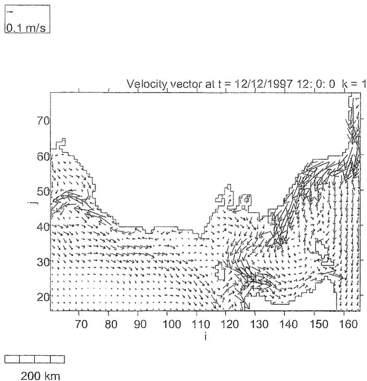
**Figure 9A.** Surface (0-5 m) current vectors predicted by hydrodynamic modelling for southeastern Australia during Cruise 2 at 12:00 h on December 12, 1997. Arrows indicate current direction; length of lines are proportional to current velocity (m/s).
