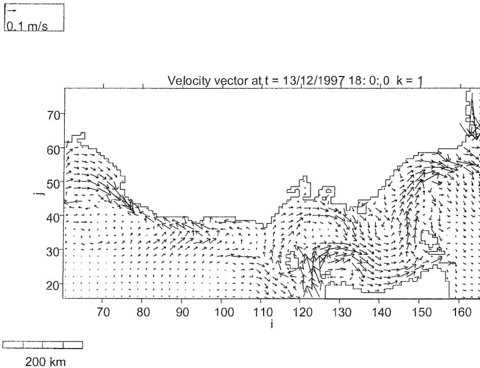
**Figure 9F.** Surface (0-5 m) current vectors predicted by hydrodynamic modelling for southeastern Australia during cruise 2 at 18:00 h on December 13, 1997. Arrows indicate current direction; length of lines are proportional to current velocity (m/s).
