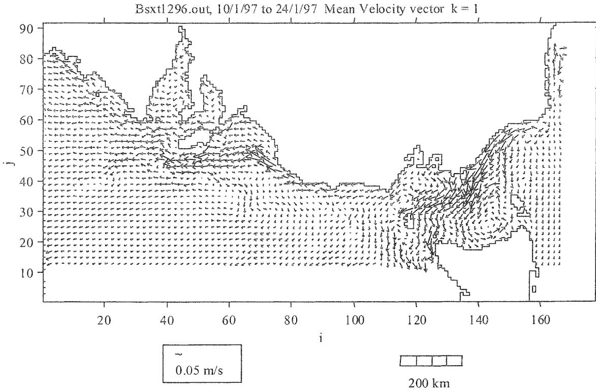
**Figure 5A.** Simulated hydrodynamic current model of southeastern Australia at a depth of 0-5 m obtained for the period 10-24 January 1997 (Cruise 1). Arrows indicate current direction; length of lines are proportional to current velocity (m/s).
