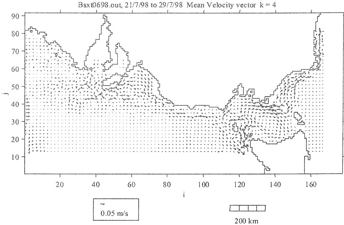
**Figure 8D.** Simulated hydrodynamic current model of southeastern Australia at a depth of 35-55 m obtained for the period 21-29 July 1998 (Cruise 4). Arrows indicate current direction; length of lines are proportional to current velocity (m/s).
