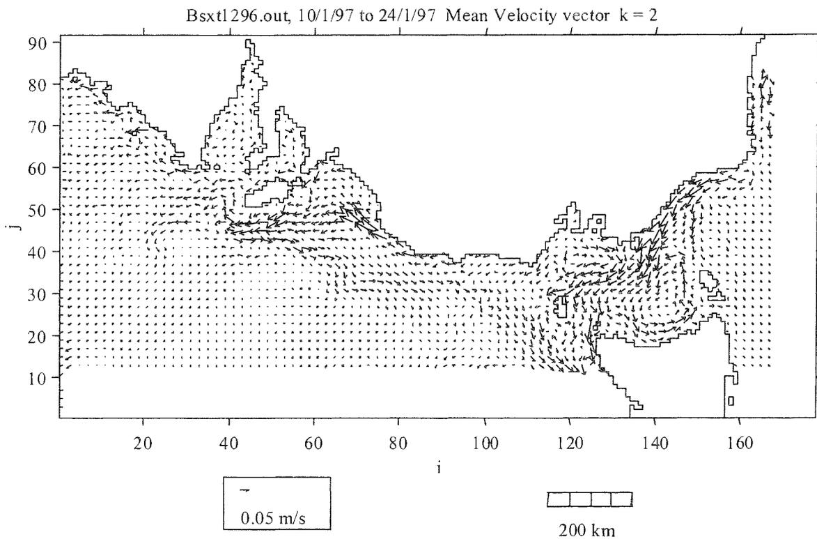
**Figure 5B.** Simulated hydrodynamic current model of southeastern Australia at a depth of 5-15 m obtained for the period 10-24 January 1997 (Cruise 1). Arrows indicate current direction; length of lines are proportional to current velocity (m/s).
