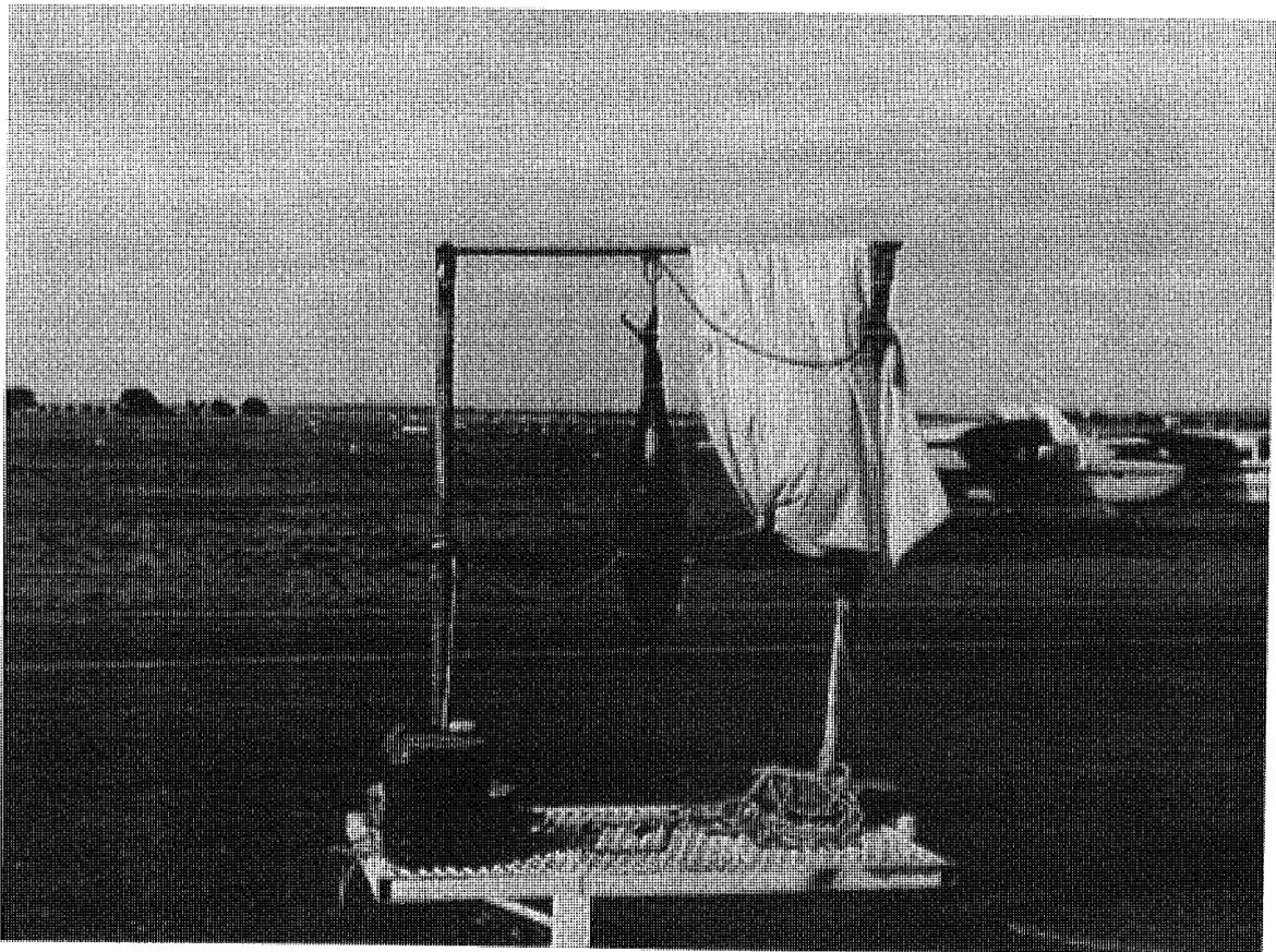
**Figure 17. Support stand for the 16kg SBT used to obtain LIDAR signature data.**
