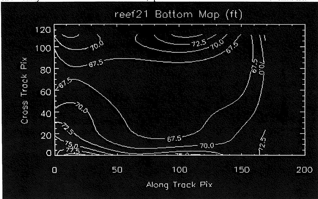
**Figure 57. Contour plot of bottom depth in the GAB for a 15 x 100m area. Depths 67-77 ft.**
