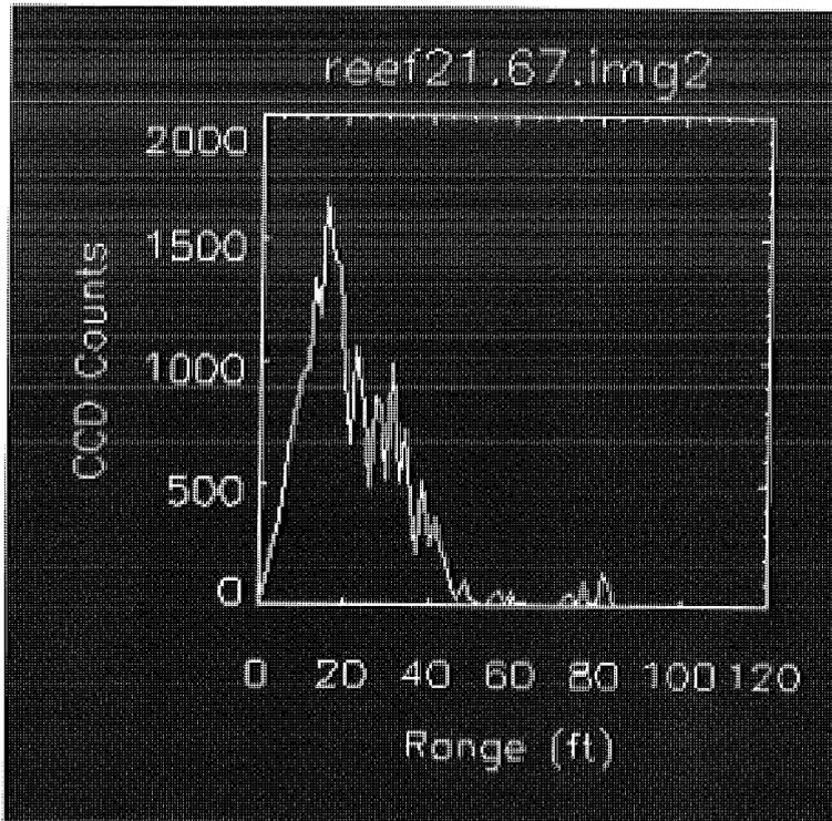
Depth slice (one column) from the greyscale raw data showed above in Figure 48. The surface return is quite obvious, but the bottom return, while discernable, is not obvious except in the filtered image. The excess noise is quite evident here.
