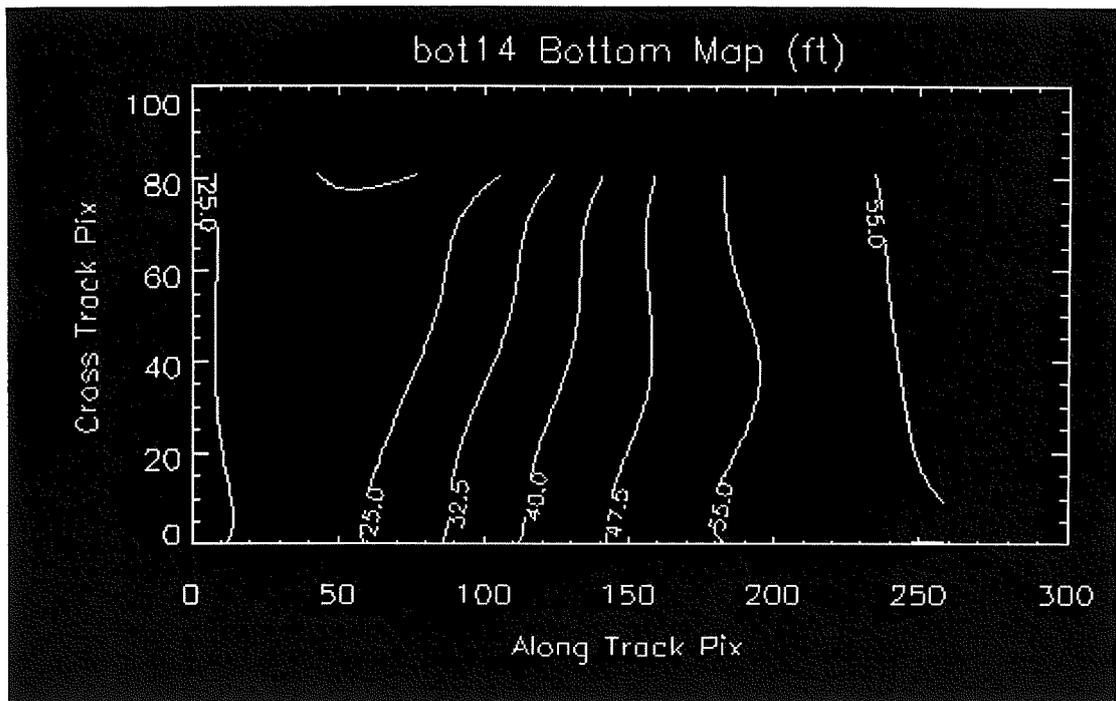
**Figure 56. Contour plot of bottom depth in Boston Bay for a 15 x 150m area. Depths 25-65 ft.**
