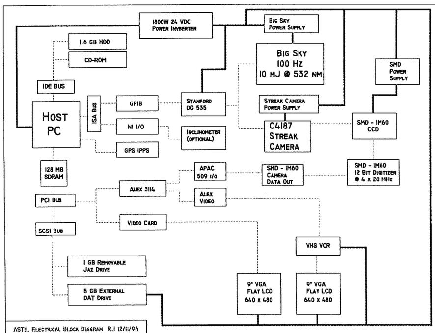
**Figure 1. ASTIL System Electrical Layout**
