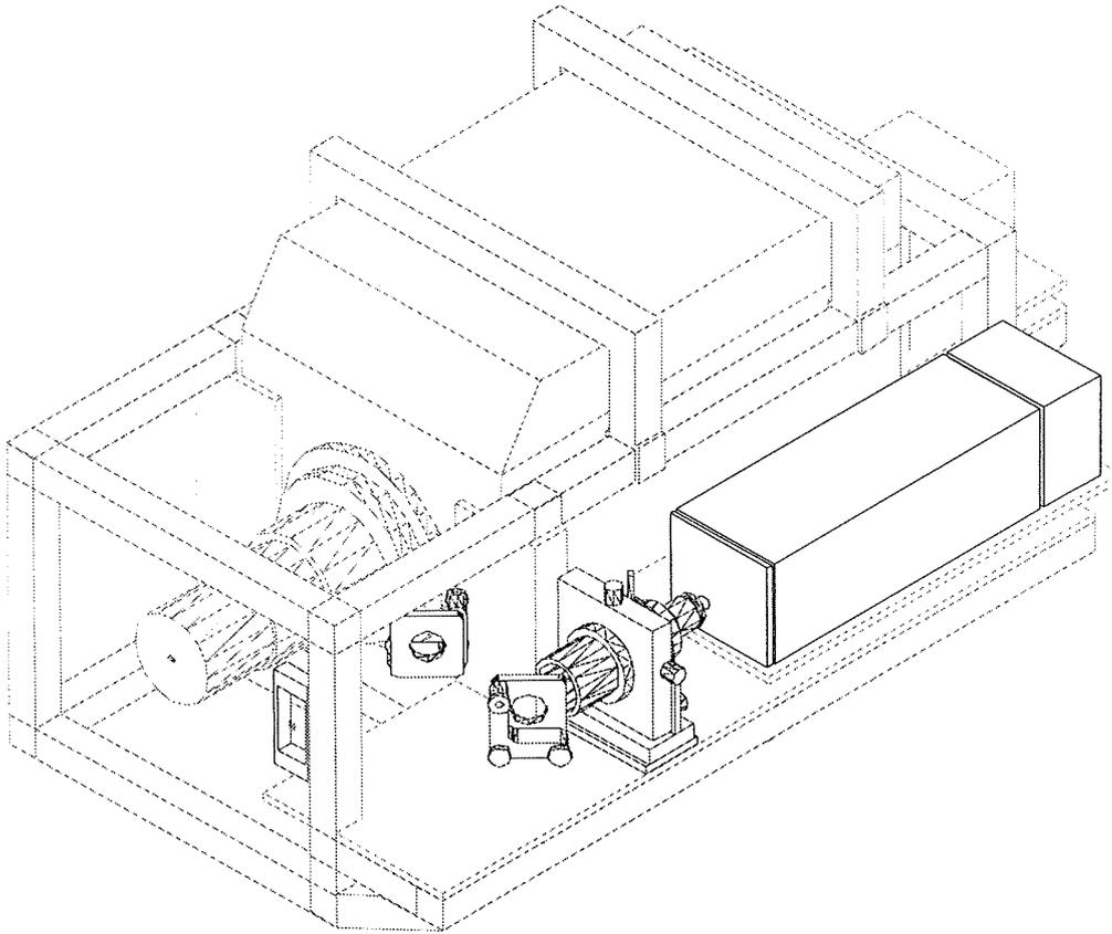
**Figure 3. Receiver/Transmitter Cage (outer rack is not shown here)**
