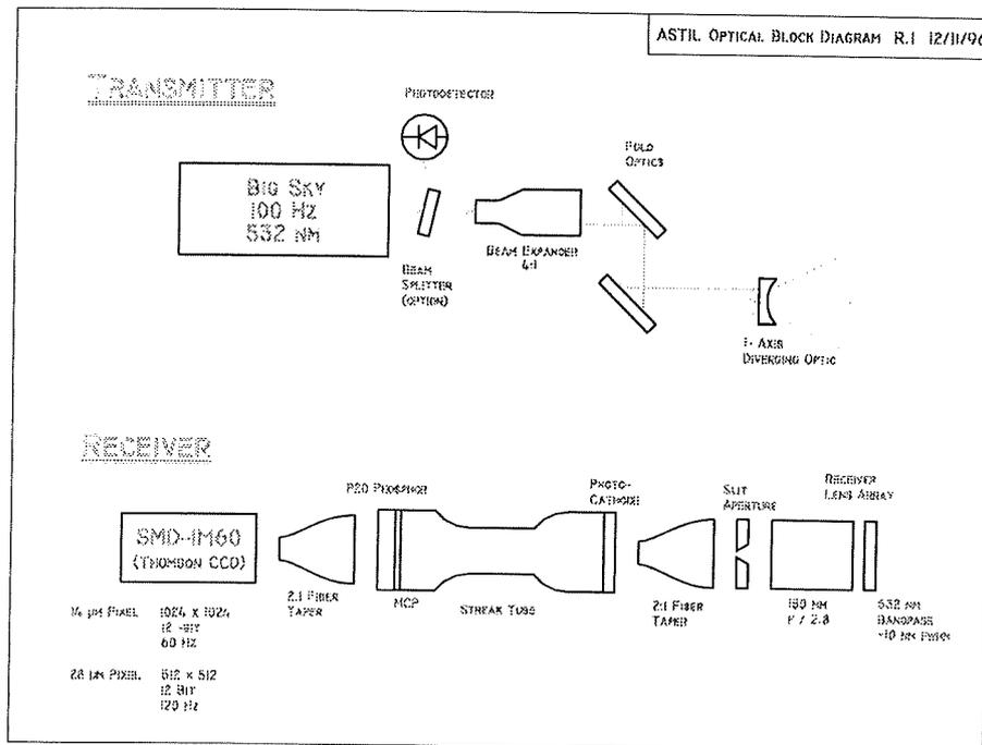
**Figure 2. ASTIL Optical Configuration**
