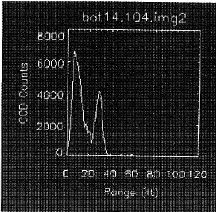
Depth slice (one column) from the greyscale raw data showed above in Figure 33. The surface and bottom returns are the obvious features in this plot.
