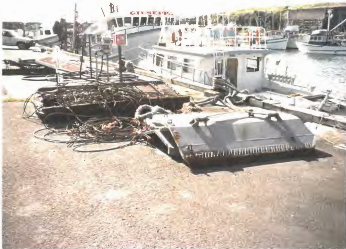
Figure 7 A pair of modern steel trawl door lying next to a pair of old wooden trawl door showing the comparison between the two types. The wooden doors were used for targeting gemfish but they have now fallen into disuse and disrepair and were not used during the current survey.
