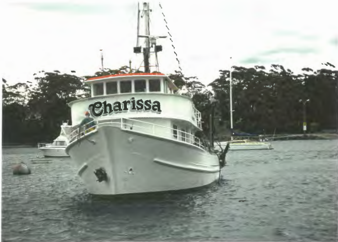
Figure 2 The survey vessel Charissa of Ulladulla. Steel vessel purpose built for gemfishing in the 1980s.
