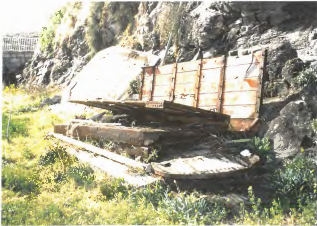
Figure 6 Old wooden trawl doors lying disused at Wollongong. These large but light wooden spreader boards were used during the peak of the eastern gemfish fishery. The light construction and large surface area caused the board to spread the mouth of the net well at low trawl speeds.
