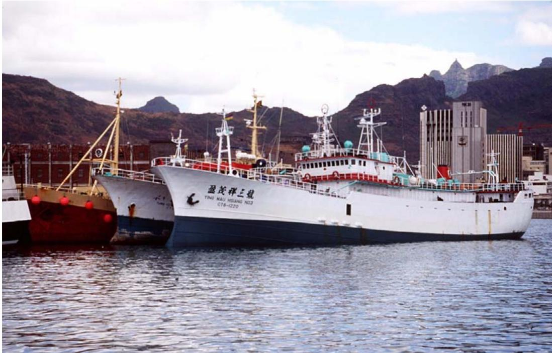
Figure 1. The Ying Hua Hsiang No 3. Tied up in Pt Louis harbour after offloading her albacore catch. The vessel is typical of the larger class of Taiwanese longliner fishing in the Indian Ocean.
