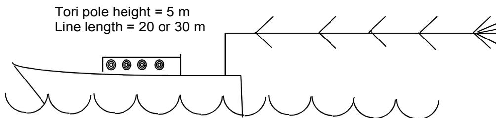
Figure 8. Drawing of tori pole and line used by some Taiwanese longline vessels in the Indian Ocean. The tip of the line does not touch the water.
