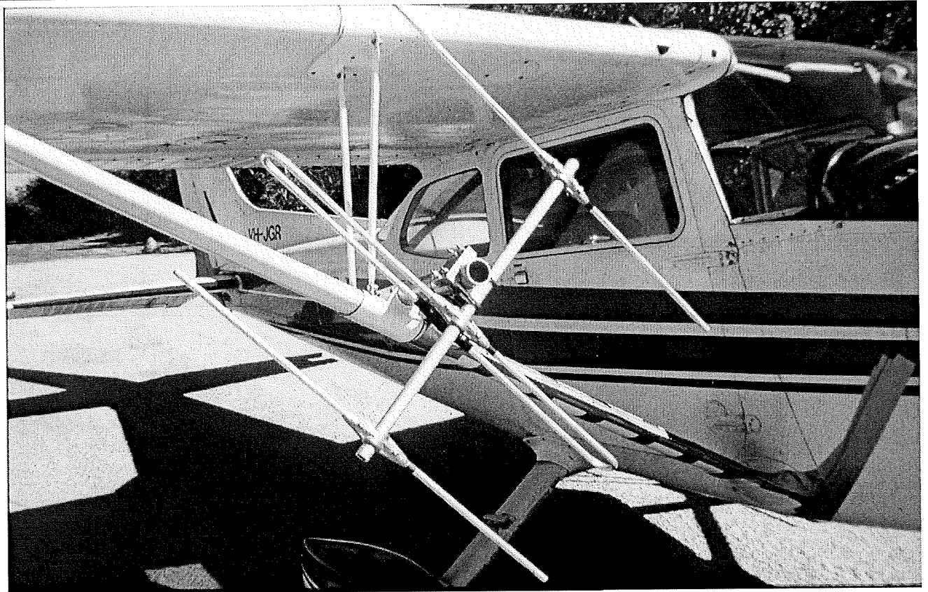
Figure 3. Photograph of starboard 3-element Yagi antennae mounted on wing strut of the Cessna 172. The antennae is directed downward at 45° and starboard of the aircraft.
