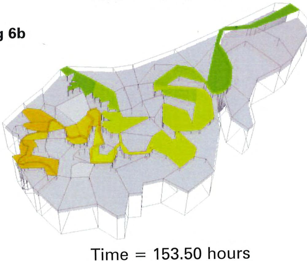
Figure 6a,b. Single frames from a computer visualisation of a ten fold increase (10x) in suspended sediment concentration in Muddy Creek during a neap tide.
