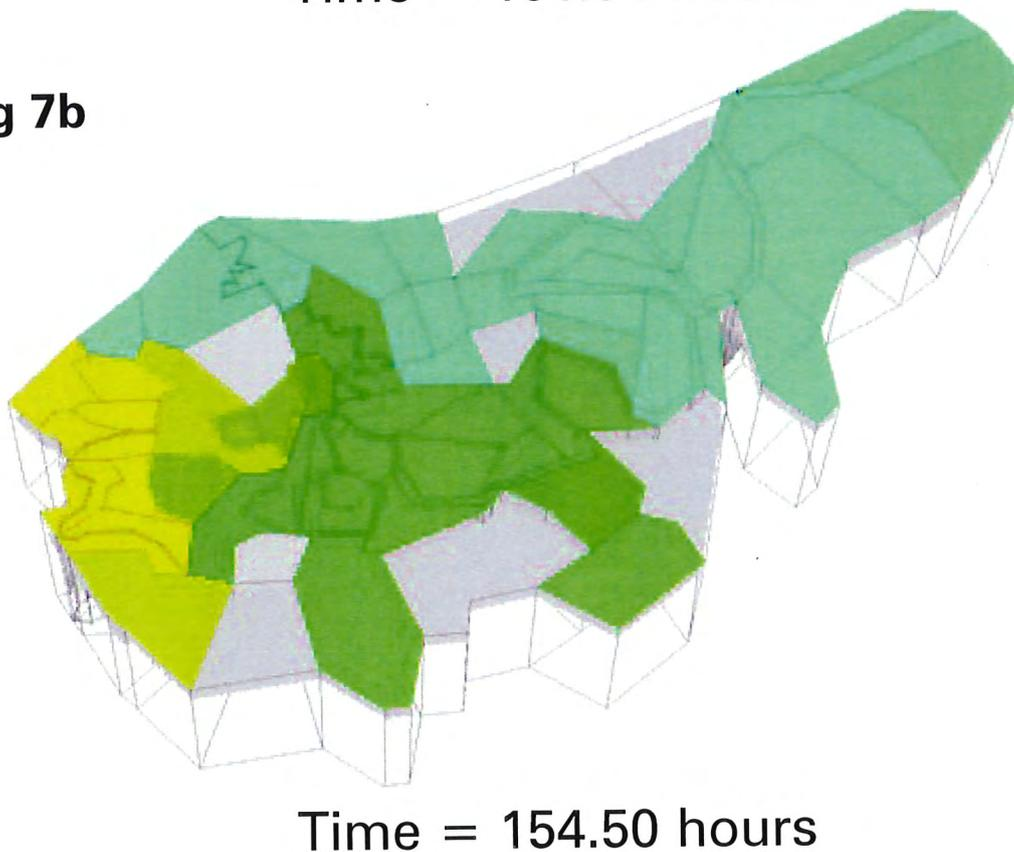
Figure 7a,b. Single frames from a computer visualisation of a ten fold increase (10x) in suspended sediment concentration in Muddy Creek during a spring tide.
