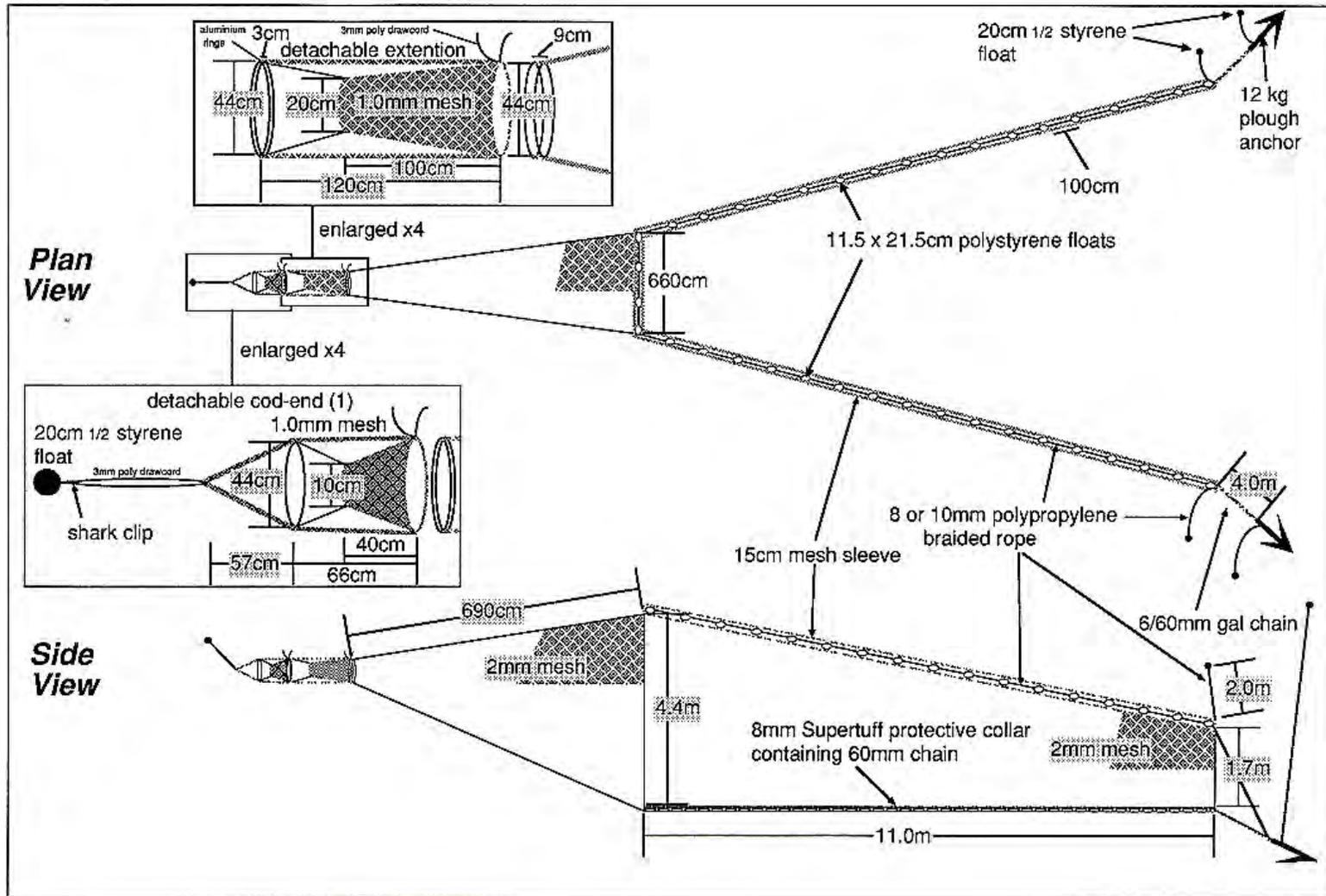
Figure 2.12 Schematic diagram of a hell net used in the study
