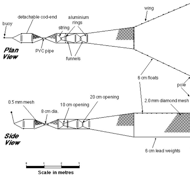
**Figure 1** Schematic diagram of a glass eel net.
