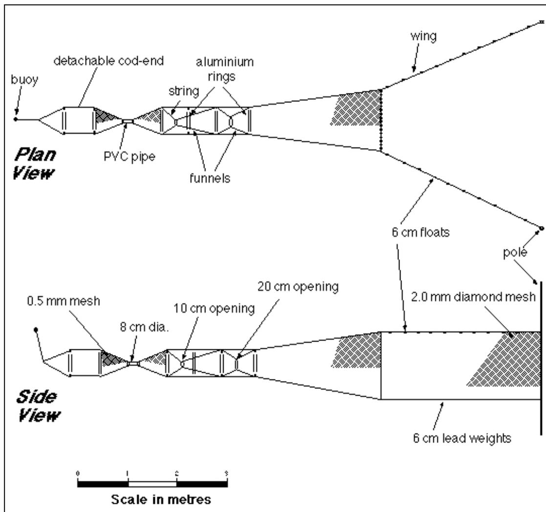
**Figure 2.11** Schematic diagram of a glass eel net used in study
