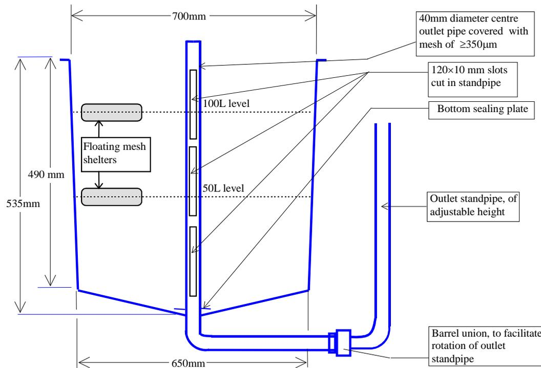
**Figure 10** Design of tanks utilised to wean and grow glass eels at Marine and Freshwater Resources Institute, Snobs Creek.
