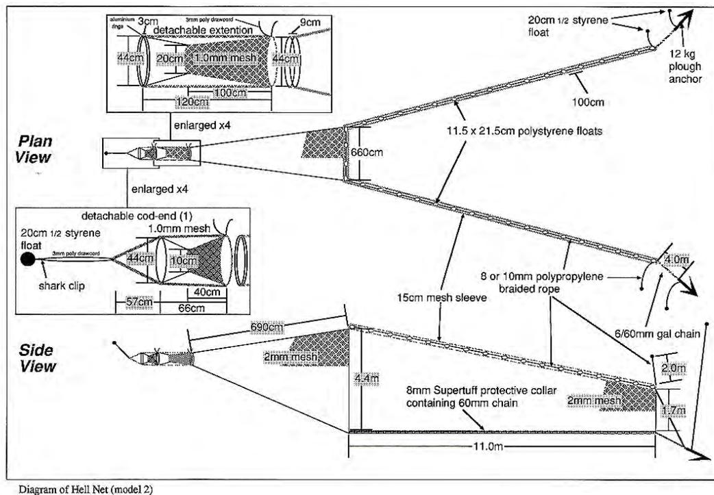
**Figure 2. Schematic diagram of hell net**
