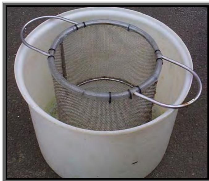
**Figure 2.14** Woven stainless steel basket design (12mm gauge frame with 3.25mm mesh).
