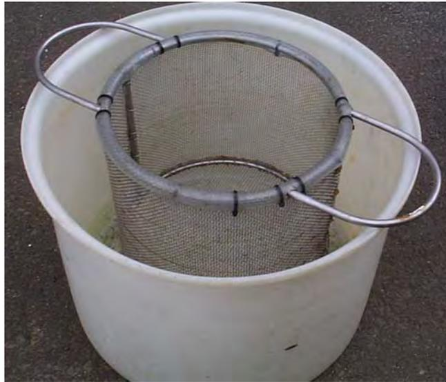
**Figure 6. Woven stainless steel basket glass eel separator (12mm frame, 3.25mm mesh).**
