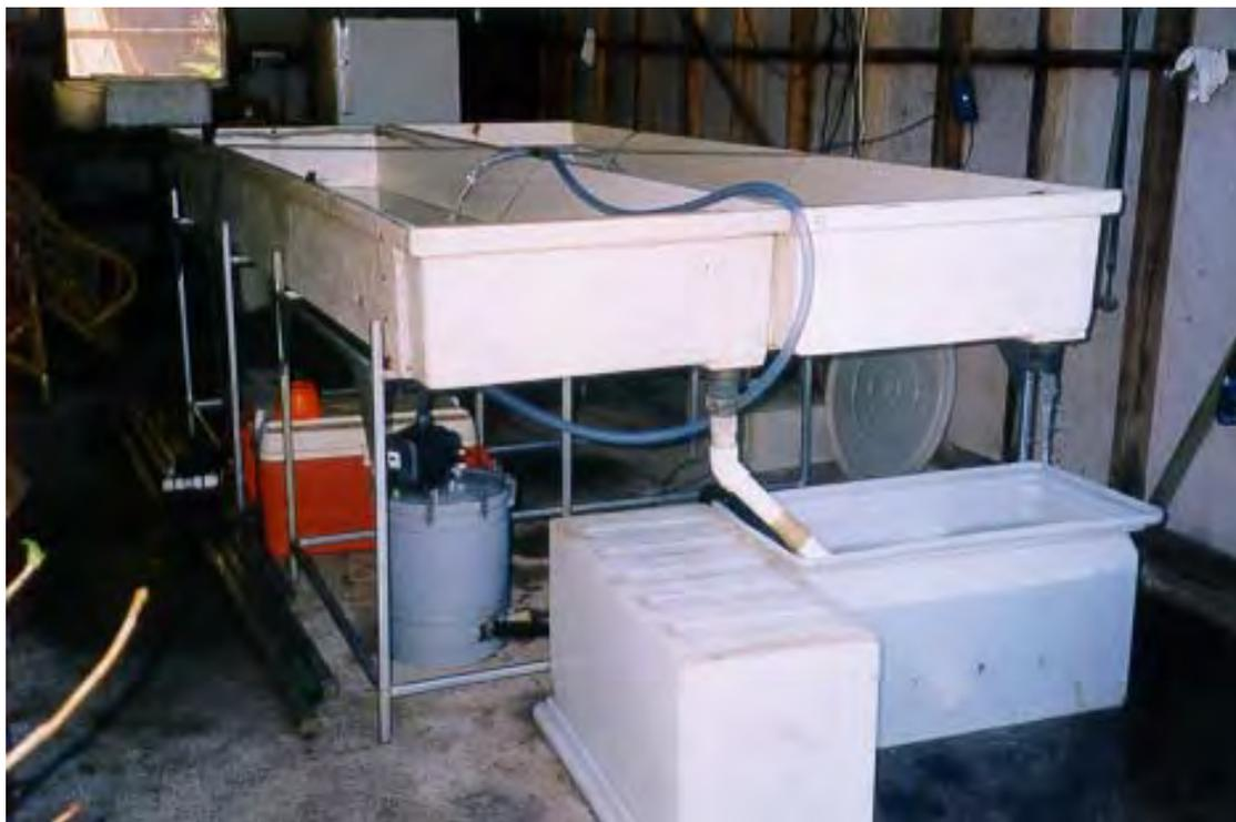
**Figure 7 Land based short-term recirculating glass eel holding facility**
