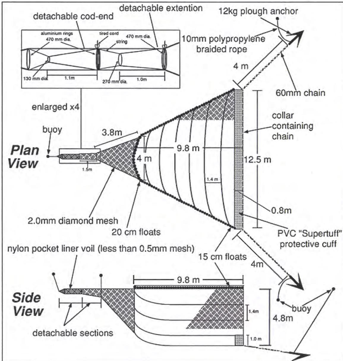
**Figure 2.13** Schematic diagram of a stow eel net used in the study.
