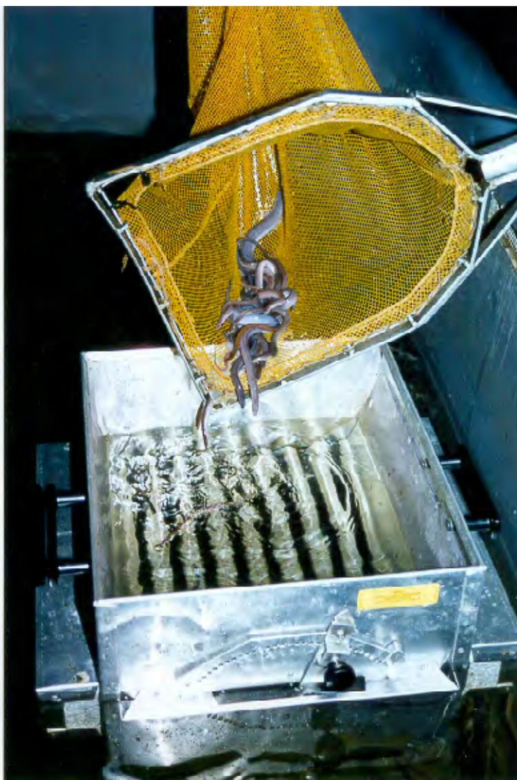
Figure 13 Mechanical grading of eels.
