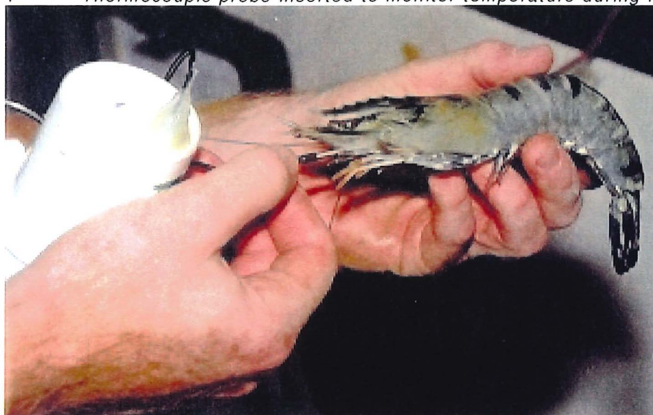
PLATE 1 Thermocouple probe inserted to monitor temperature during freezing
