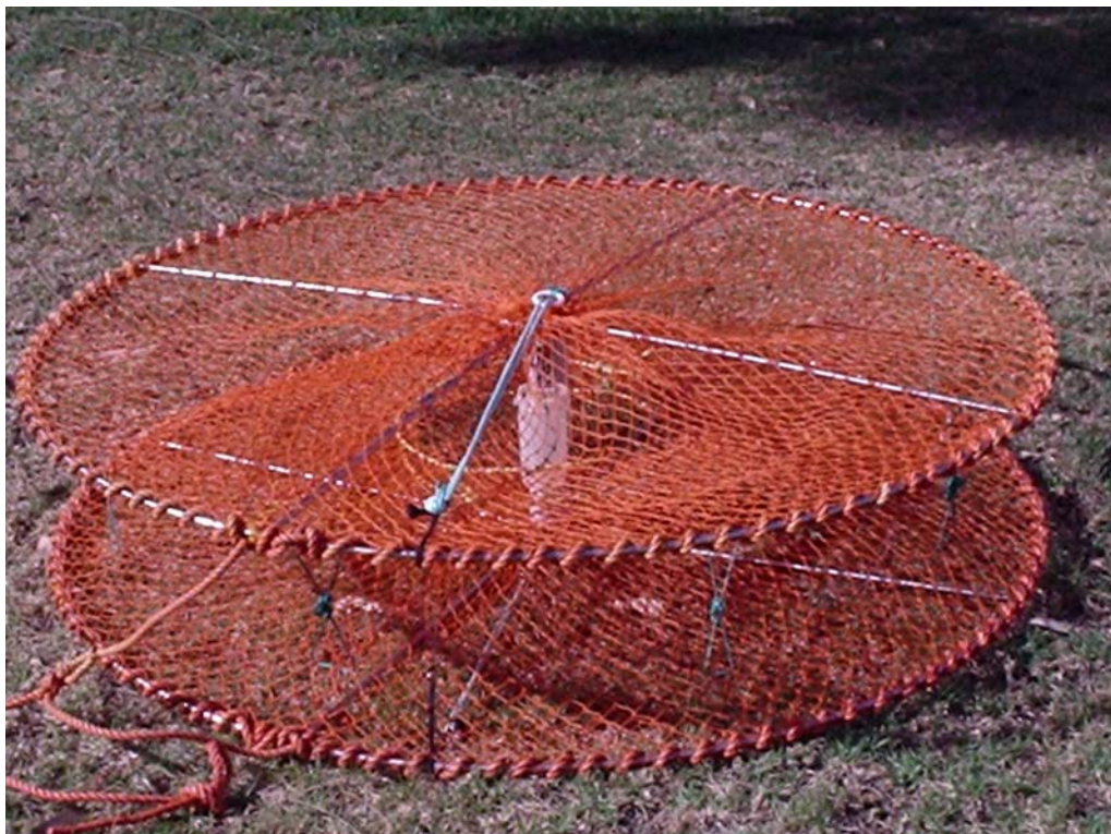
Figure 10. Research crab pot with a mesh size of 55 mm (from Svane and Hooper, 2004).
