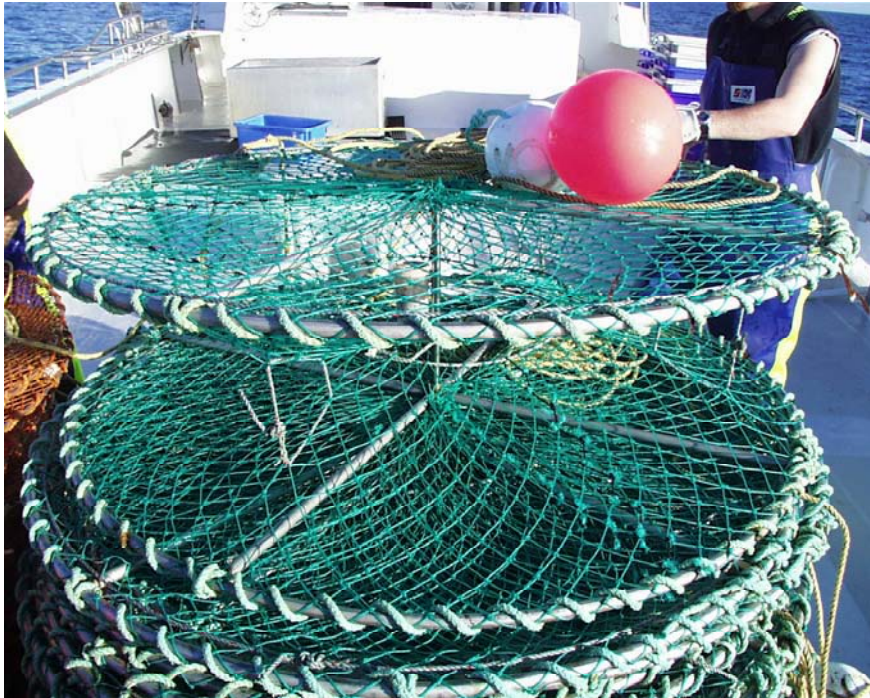
Figure 6. Commercial crab pot as used by the fishery with a mesh size of 90 mm (from Svane and Hooper, 2004).
