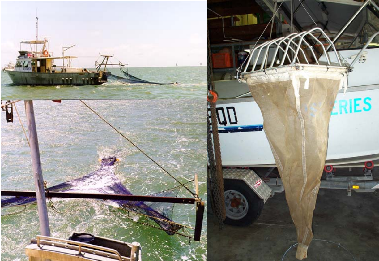
Figure 8.2 FRV Warrego showing the 5 m beam trawl used to sample juvenile blue swimmer crabs. Plankton net showing grid used to exclude large jellyfish from entering the net.
