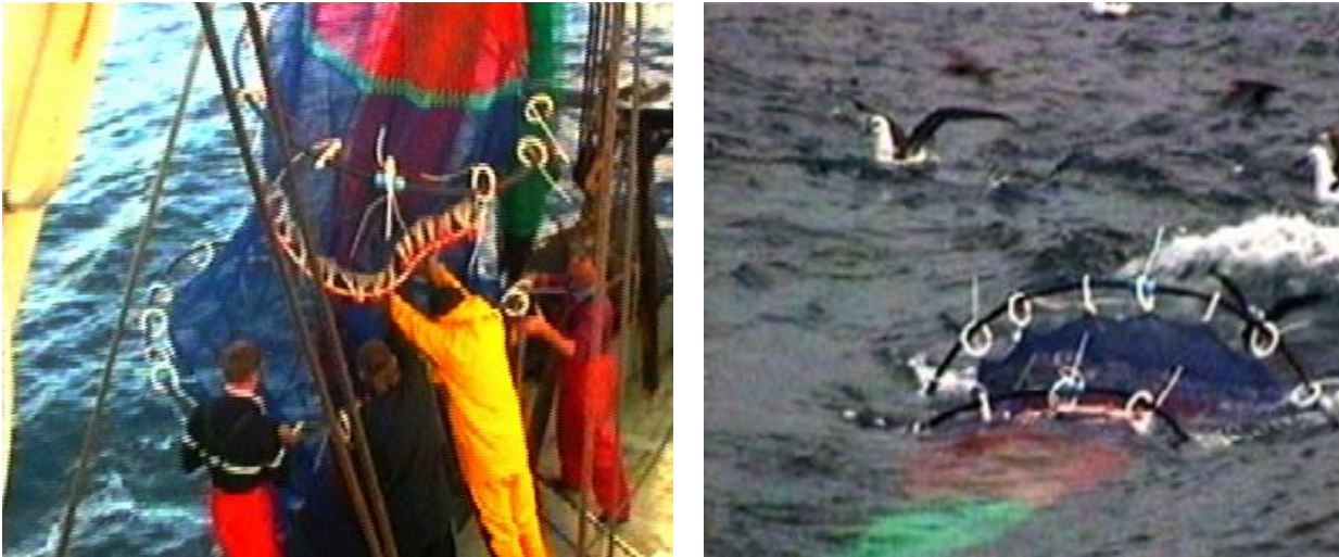
Plate 5-2. Setting and deploying the covered codend on the Shelley H during project field trials.
