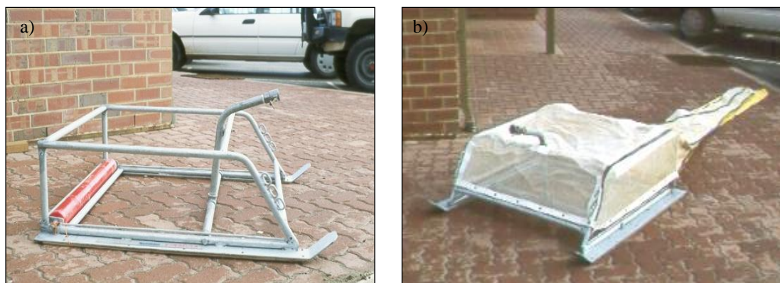
Figure 5.2. Water-jet net design showing (a) the galvanised frame without netting and (b) with net attached.
