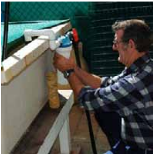
Figure 35 Nursery tank filter element being changed.
