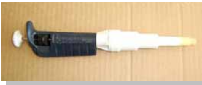
Figure 22 Sampling of eggs using an automatic pipette (above) and placing them into small weighing boats (right) for counting by eye or with the aid of stereo microscope at low magnification
