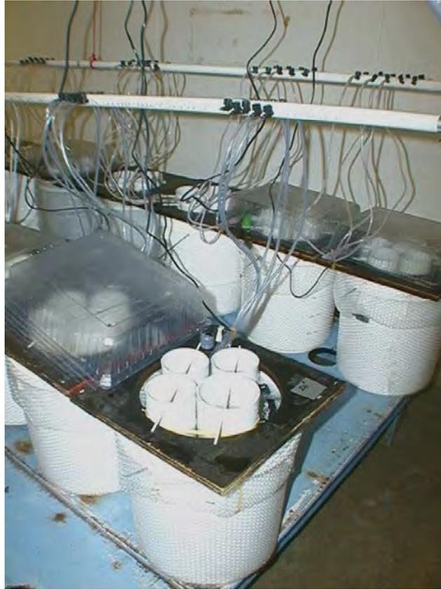
**Plate 1.** Experimental array showing some of the 20 temperature bath/seawater reservoirs housing 4 mini-downwellers that in turn each accommodated a replicate of the four discrete age/size classes of juvenile *H. rubra*.
