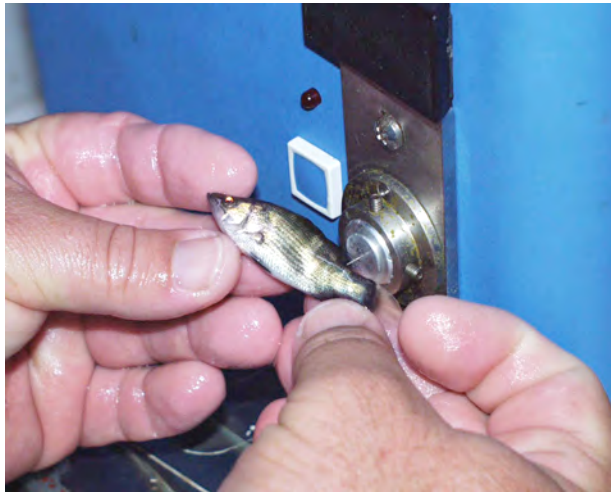
Figure 2.3 Tagging a barramundi with a coded wire tag (Photo Mark Dawson).
