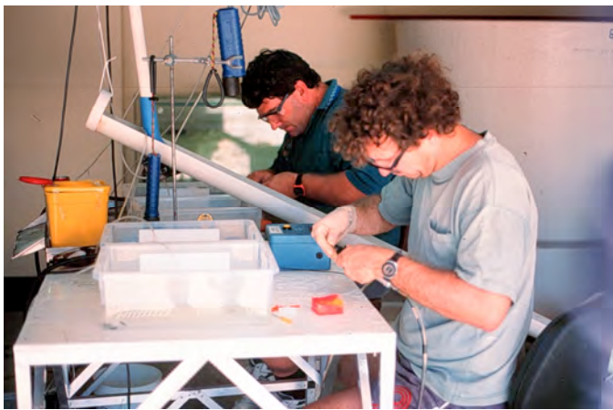
Figure 2.2 VIE tagging set up. Note two taggers in operation, containers for anaesthetising fish and chute down which tagged fish travel to a recovery tank (Photo M. Hutchison).
