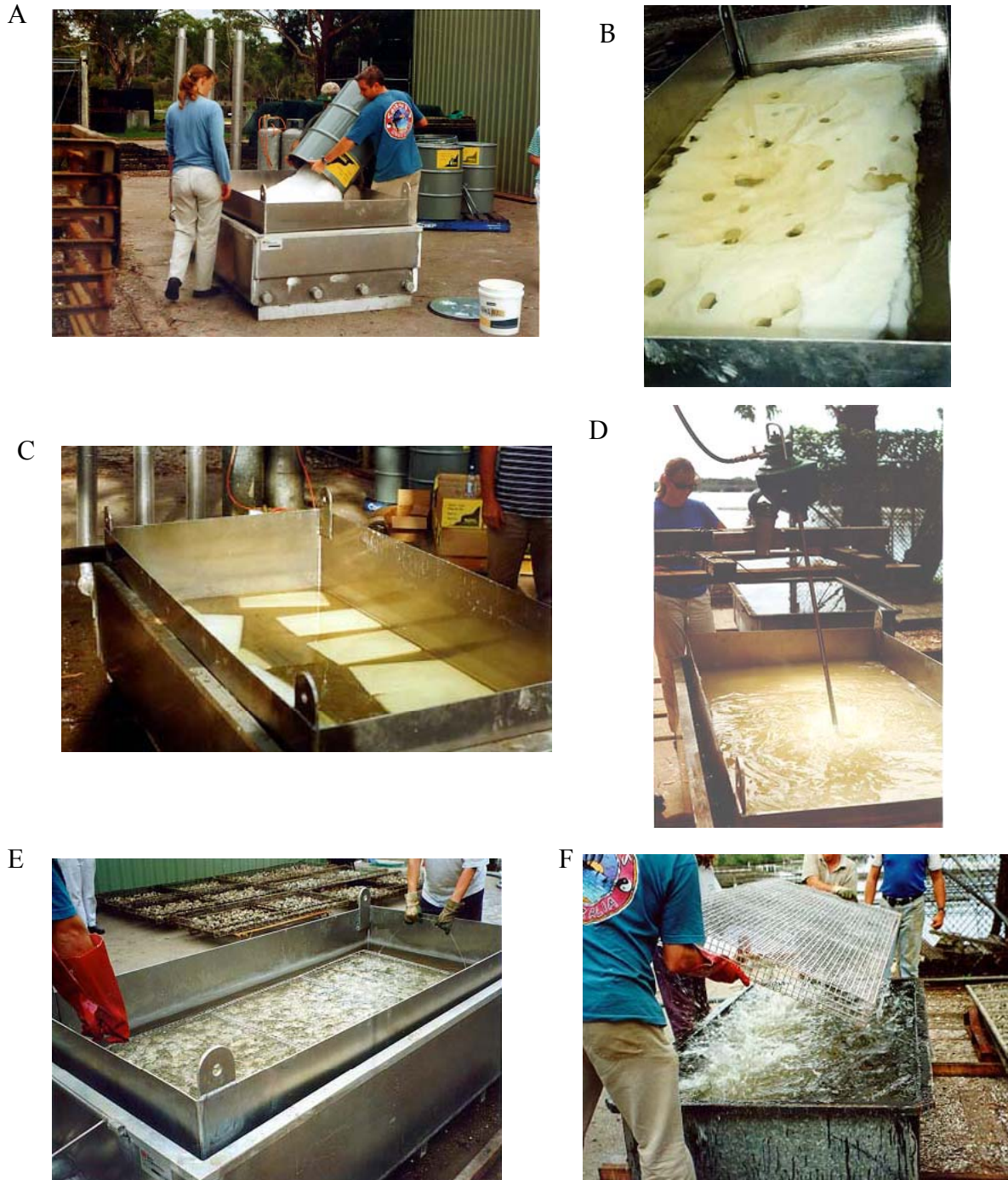
Figure 1. The coating application process in the Commercial trial at Port Macquarie. Adding OysterClear Original to the stainless steel bath housed in a gas-heated water jacket (A); Melting Original (B); Melting blocks of OysterClear coating 2 (C); mixing Coating 2 with a high speed disperser mounted on a fork lift (D); dipping oysters in a tray into Original; transferring coated oysters into cool water (F).
