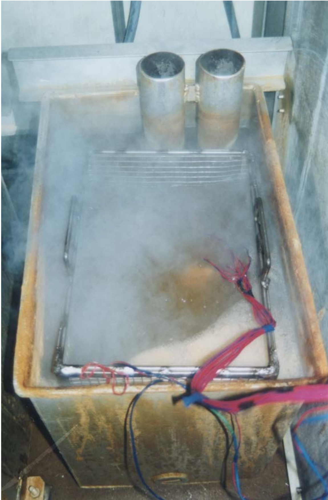
Prawns with thermocouples attached being cooked by boiling in a commercial prawn cooker.
