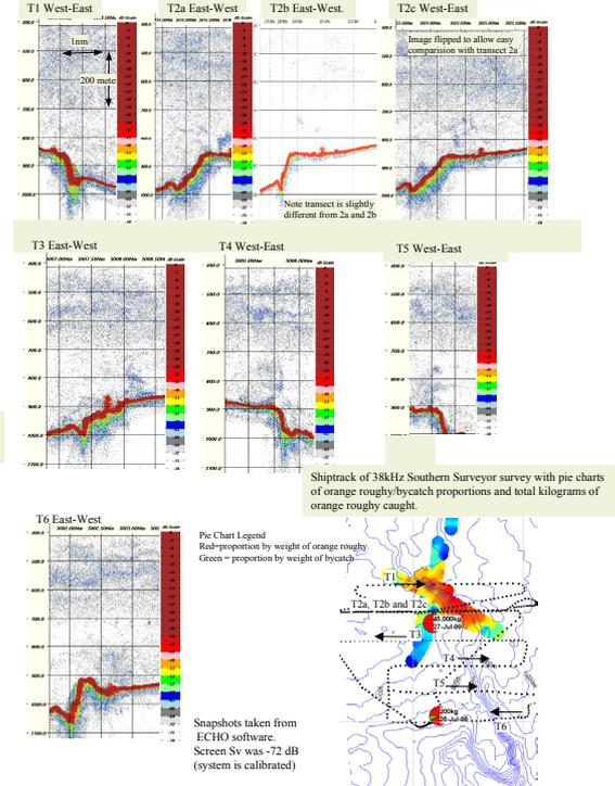
c) Southern Surveyor vessel mounted 38kHz echosounder data. Survey 3
