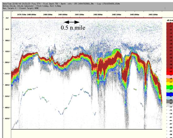
38kHz echogram from East to West transect over the main aggregation. MUFTI Depth 600 metres
