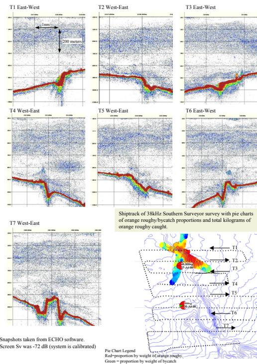
d) Southern Surveyor vessel mounted 38kHz echosounder data. Survey 4
