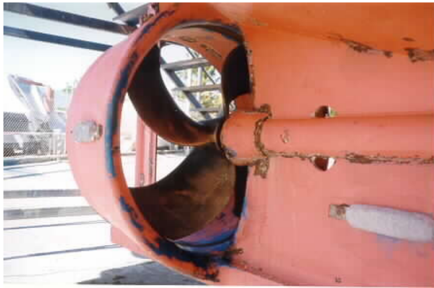
Figure 5.4.3 Propeller with nozzle, from Queensland east coast trawler.
