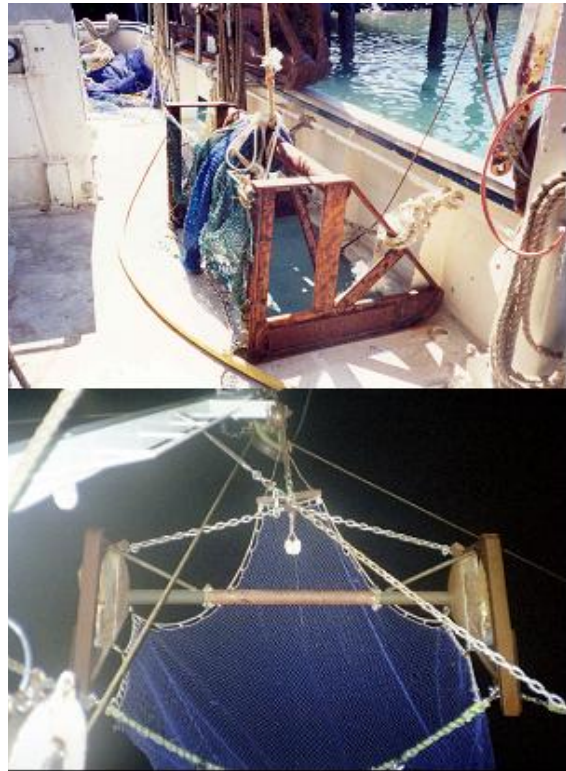
Figure 5.4.5 Beam trawl try gear on board vessels in the eastern king prawn fishery.
