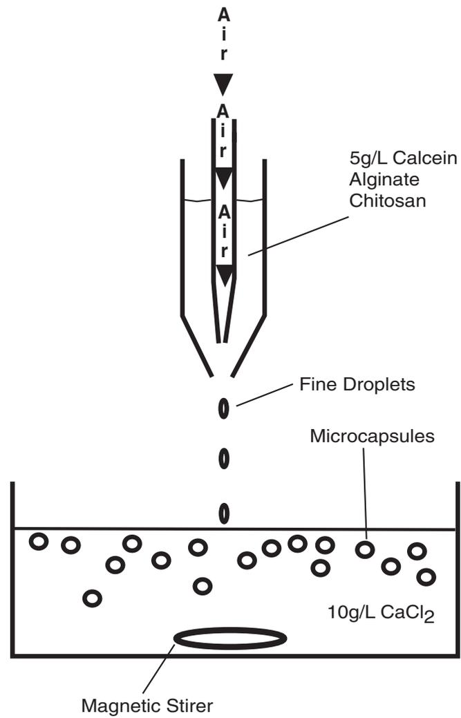
**Figure 6.** Shows the procedure and apparatus used in the preparation of calcein microcapsules that were mixed with food and fed to an number of *Sardinops sagax* held in a sea cage.
