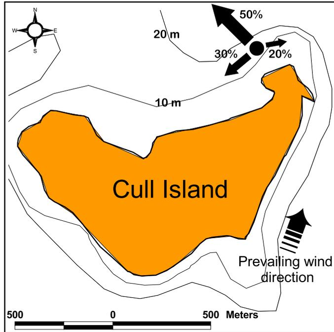
**Figure 7.** Cull Island, Esperance, showing the location of the anchoring position, the prevailing wind direction, the frequency of the three most common directions that the net hung from the anchored vessel and the bathymetry adjacent to the island.
