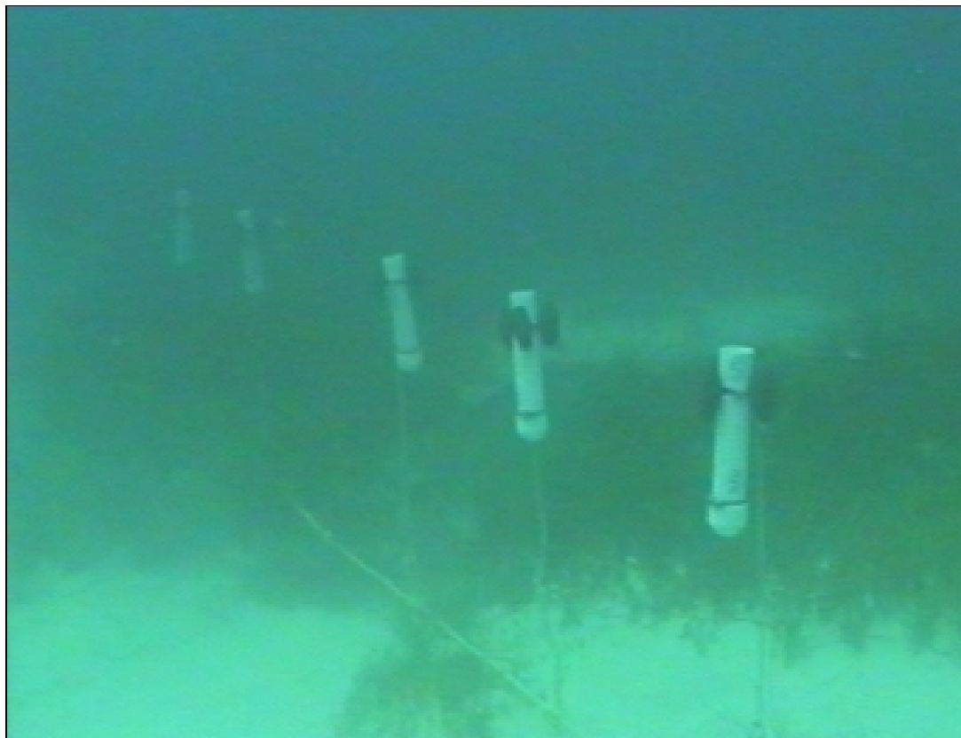
Figure 5.18 Sediment traps used for the study of organic deposition
