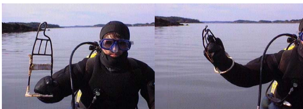
Fig A4.3.1 Purpose-designed harvesting rake for sea urchins (New Brunswick, Canada)
