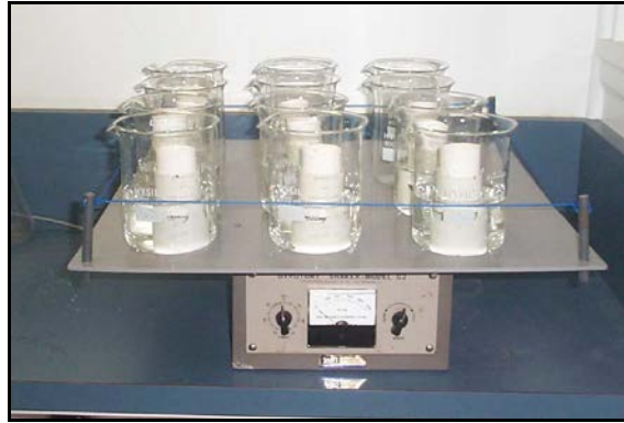
Figure 24. Shaker table used to determine the water stability of heat-treated diets.
