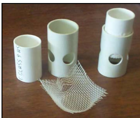
Figure 23. Screens used for determining water stability of heat-treated diets.
