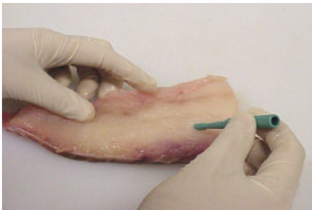
Plate 14.3. Biopsy tool used for sampling fish flesh.
