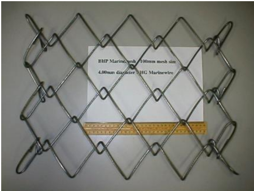
Figure 3 : Onesteel 100mm mesh, 4mm diameter
