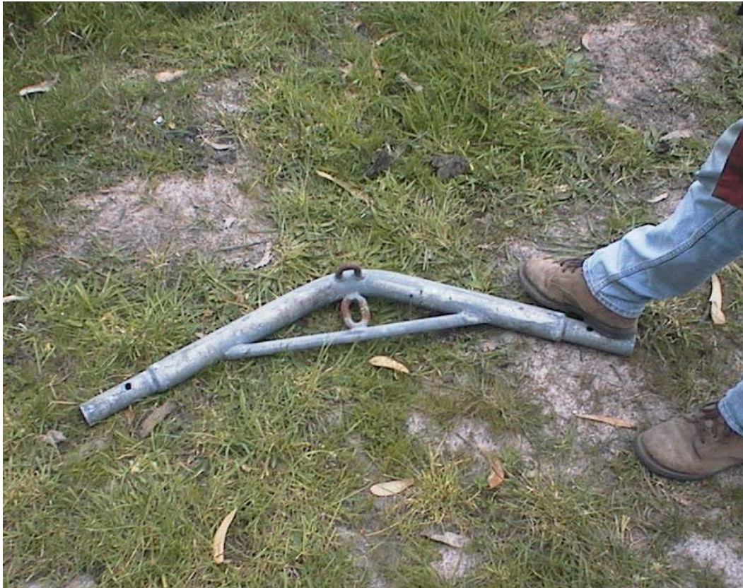
Figure 24 : Corner section of trialed lightweight sinker ring
