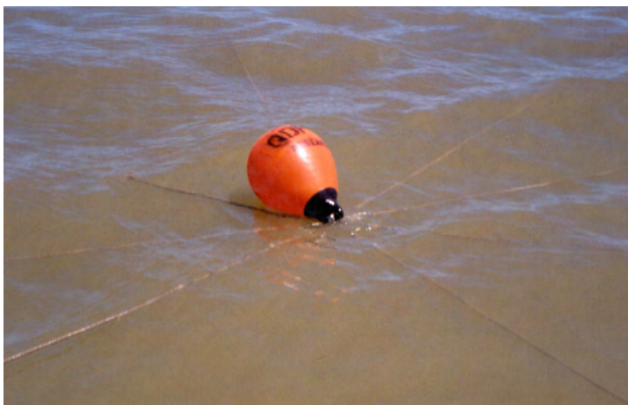
Figure 36. The trapping web layout showing the centre buoy and the eight arms attached
