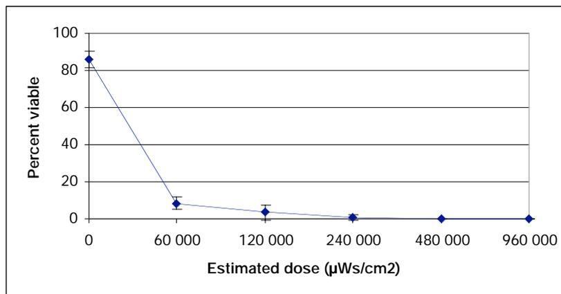
Fig. 2. Effects of cumulative dose of ultraviolet light on the viability of hypnospore stages of *Perkinsus olseni*, placed into the periodically inverted inlet tube with seawater. Bars represent standard deviations.
