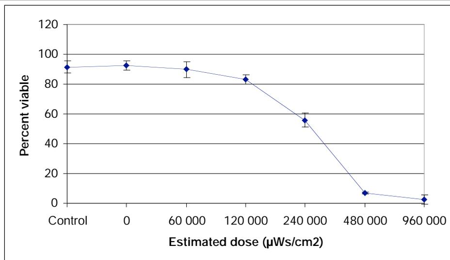
Fig. 1 Effects of ultraviolet light exposure on the viability of *Perkinsus olseni* hyphospores, placed into the inlet tube of the LC 20 UV unit with seawater. Bars represent standard deviations.
