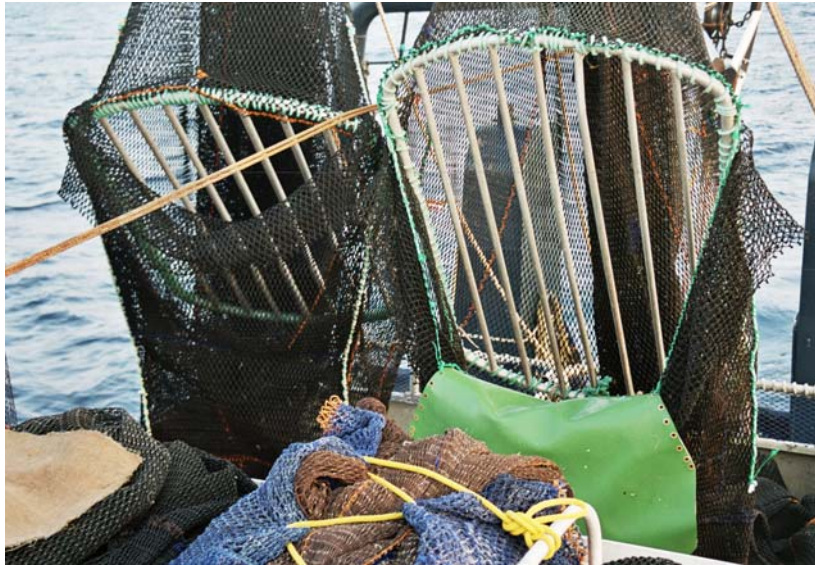
Figure 12-13. Both TEDs shown above are identical in construction, with the exception of the canvas section attached to the TED on the right. However, the TED on the right has lost grid angle and the escape cover is severely stretched (large gaping opening). Prawn loss was high from this TED and it requires substantial maintenance (i.e. re-set grid angle and replace escape cover). The TED on the left is new and ready for operation.
