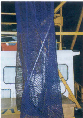
Figure 6: The grid at the top lost substantial amounts of prawn due to problems associated with a low grid angle (25°), including a loose fitting escape cover (brown netting). The same grid (lower) was re-hung at a greater angle (45 – 50°) and actually caught more prawns than a standard net. Note how the lower grid expands the shape of the codend (the codend has not yet been fitted to the TED); this indicates an appropriate grid height for the selected grid angle
