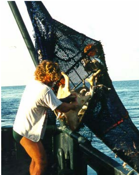
Figure 12-11. Small escape openings can cause grid obstructions that often result in catch losses.
