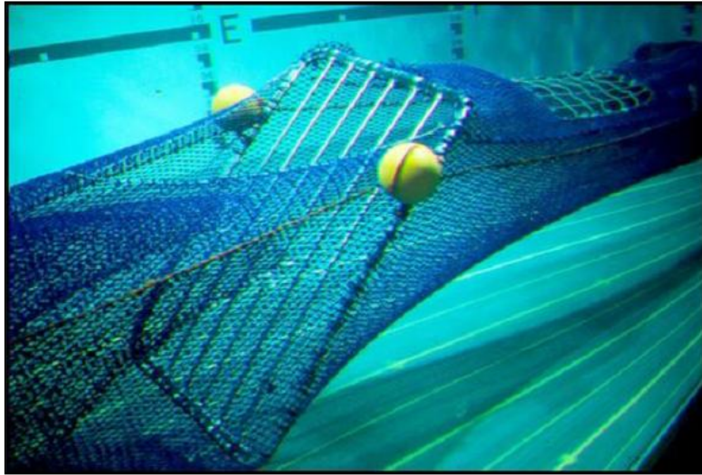
Figure 10-1. An example of a legal codend (TED + BRD) used in the NPF. Note the presence of both the TED (Nordmore grid), and behind it, the BRD (Square-mesh panel). Photo taken at the AMC flume tank.
