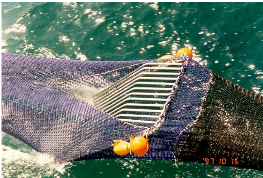
Figure 12-5. The AMC designed NAFTED shown here was a rectangular grid designed with a bar spacing of 60mm. Note that this version of the TED had no escape cover and the width of the escape opening was equivalent to the width of the grid.
