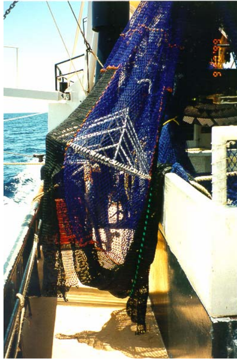
Figure 12-8. A pyramid TED with escape covers (black mesh) extending over both escape openings.
