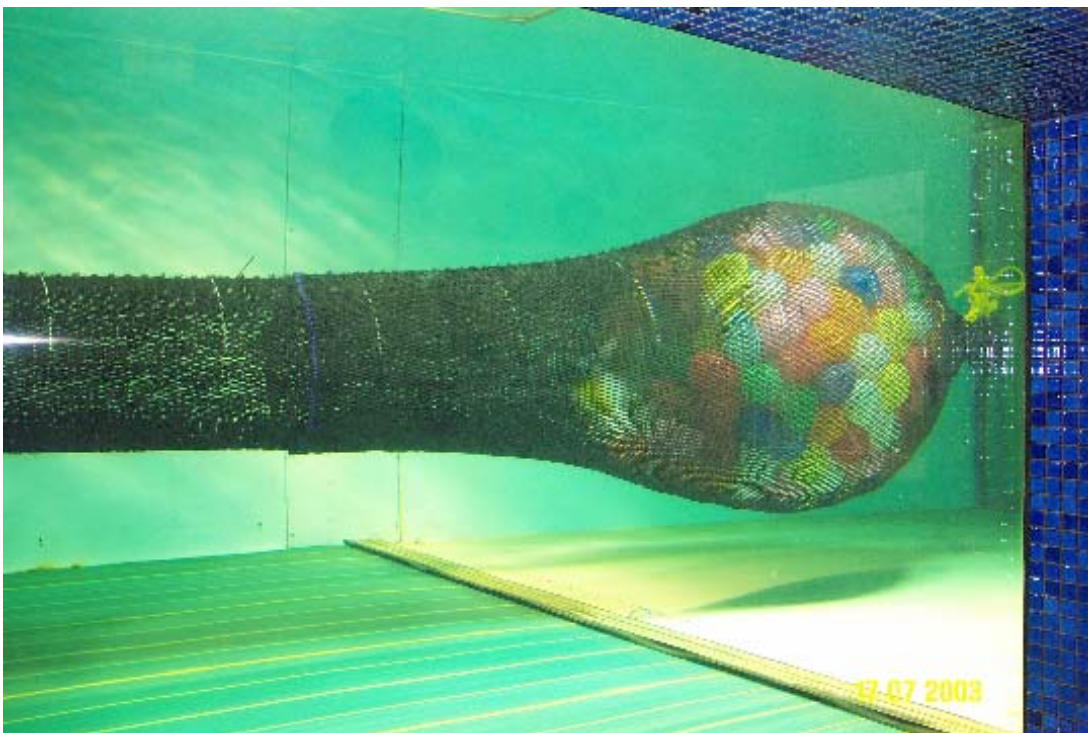
Figure 13-5. Catch was simulated with 350 x 2kg water filled balloons.
