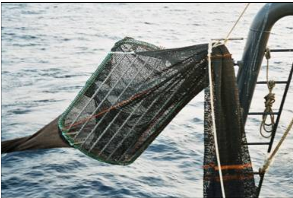
Figure 9-2. Example of TED showing position of installation in net. (Photo- G. Day)
