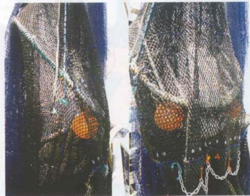
Figure 8: The TED on the left was losing substantial amounts of prawns when first installed by the crew. In an attempt to reduce this loss they lengthened the escape cover and added chain and lead weights (right photo). These modifications only served to increase grid blockage by sponges with a resulting increase in prawn loss. The initial problem was not related to a poor escape cover, but to an under-sized grid and low grid angle (left photo). The grid was reinstalled at a higher angle by the author and an escape cover without weights was used extending only 6 meshes past the TED frame. Catch loss was eliminated and the incidence of grid blockage significantly reduced
