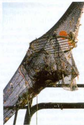
Figure 5: Oval-shaped grids conform well to the shape of the codend during operation. Note that the escape opening extends part way around the sides of the grid
