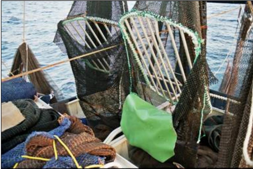
Figure 9-1. Examples of TEDs used on one of the Observer fleet vessels. (Photo- G. Day)
