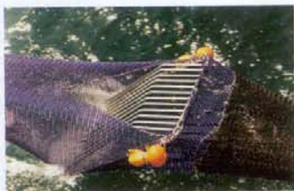
Figure 4: The AMC designed NAFTED is an example of a rectangular bent-bar grid. Note that the width of the escape opening is equivalent to the width of the grid. This version of the NAFTED has no escape cover and was designed with a bar spacing of 60mm to exclude large jellyfish
