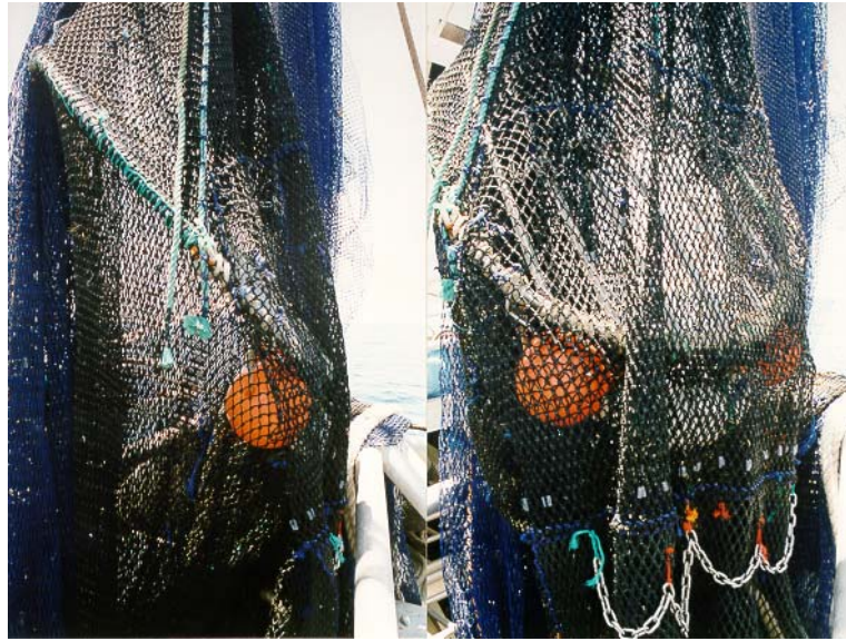
Figure 12-14. This TED was losing substantial quantities of prawn when first installed by the crew. In an attempt to reduce this loss they lengthened the escape cover and added both chain and lead weights (right photo). These modifications only increased the problem of grid blockage with sponges, and prawn loss was further increased. The initial problem was not related to a poor escape flap, but to small a grid and a low grid angle (left photo). The grid was reinstalled at a higher angle by the author and an escape cover without weights was used extending only 6 meshes past the TED frame. Catch loss was eliminated and the incidence of grid blockage significantly reduced.
