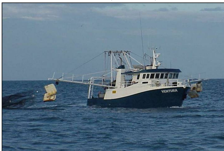
Figure 9-6. Typical NPF trawler using twin-rigged otter trawls. (Photo – Q. Dell)
