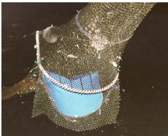
Figure 6-7. Canvas sheet attached to bottom of codend to facilitate the passage of sponges and debris from the trawl.
