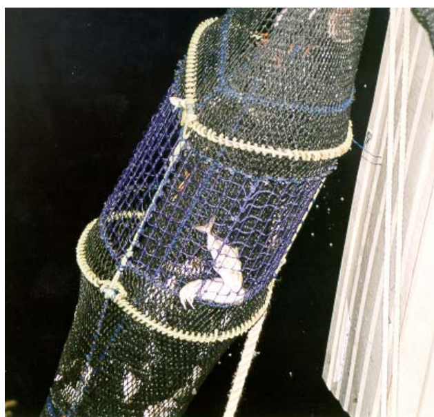
Figure 6-2. The full RES with square meshes extending radially around the entire codend circumference.
