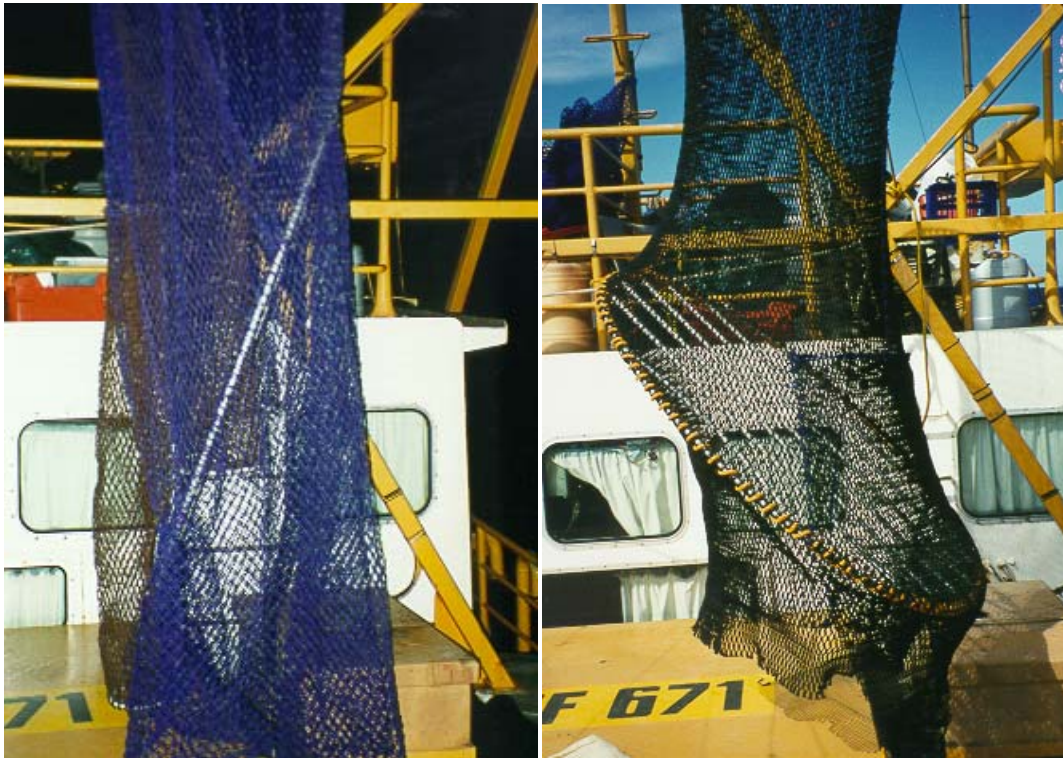
Figure 12-10. The grid on the left lost substantial amounts of prawn due to problems associated with a low grid angle ( 25^\circ ). The same grid (right) was re-hung at a greater angle ( 45 - 50^\circ ) and actually caught more prawn than a standard net. Note the poor contact of the escape cover (brown netting) with the grid at the low grid angle compared to the higher angle. Also note how the grid on the right expands the shape of the codend; this indicates an appropriate grid height for the set angle.
