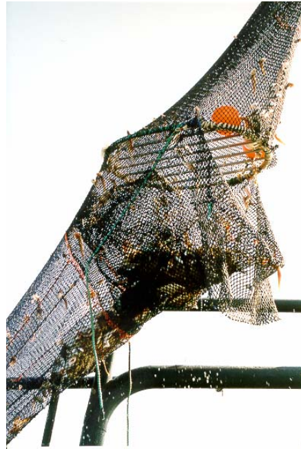
Figure 12-6. Oval-shaped grids conform well to the shape of the codend during operation. Note that the escape opening extends part way down the sides of the grid frame.
