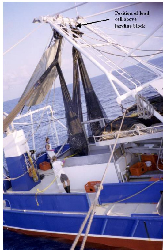
Figure 7-1. Deck layout showing position of load cell above lazyline block. (Photo- Q. Dell)
