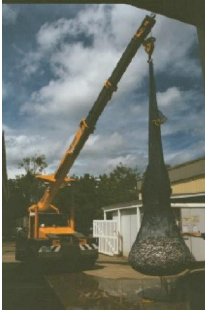
Figure 7-4. A codend being calibrated with known weights of small bycatch (CSIRO, Cleveland, Qld).
