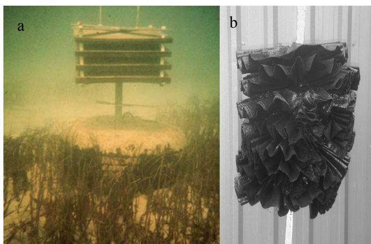
**Figure 41.** a) Crevice collector b) Bottlebrush collector
