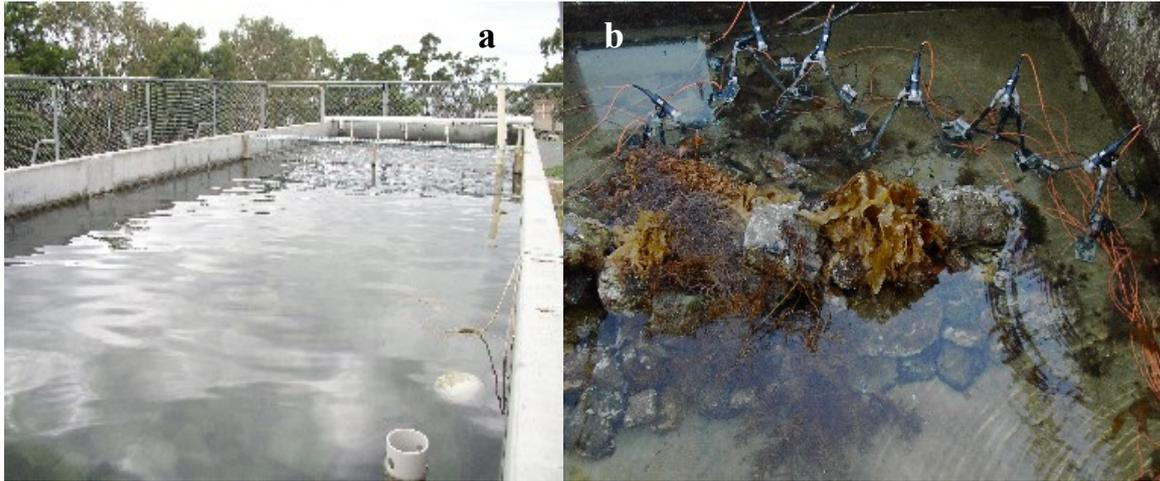
**Figure 27.** a) Raceway tank in which the mesocosm reef was constructed. The divider can be seen towards the far end of the tank b) mesocosm reef with water level lowered to allow thorough searching of the reef – cameras and lights can be seen deployed for this trial.
