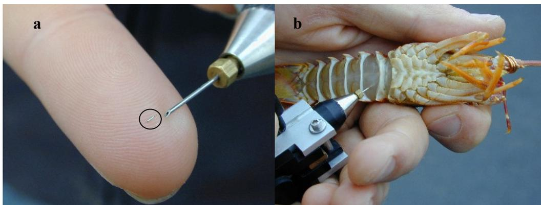
**Figure 14.** a) Coded microwire tag (on finger) and applicator needle b) Injecting coded microwire tag into juvenile lobster.
