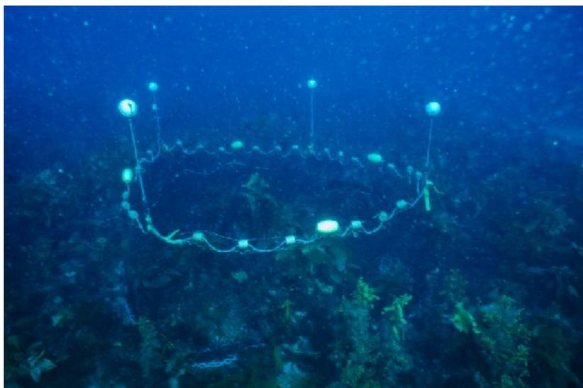
**Figure 50.** Deployed mesh cage. While the cage mesh is not visible, the floats at the top of cage walls can be seen, as can the chain ensuring that lobsters are unable to escape under the cage walls and predators are unable to get into the cage area (Photo by Hugh Perderson).
