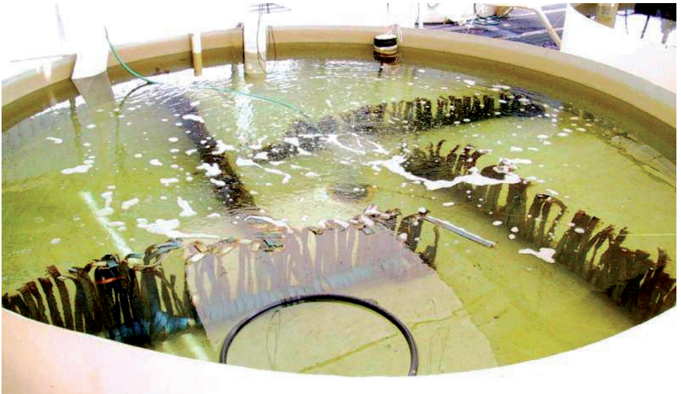
Figure 49. Arrangement of Aquamats in the experimental tank for Treatment B.
