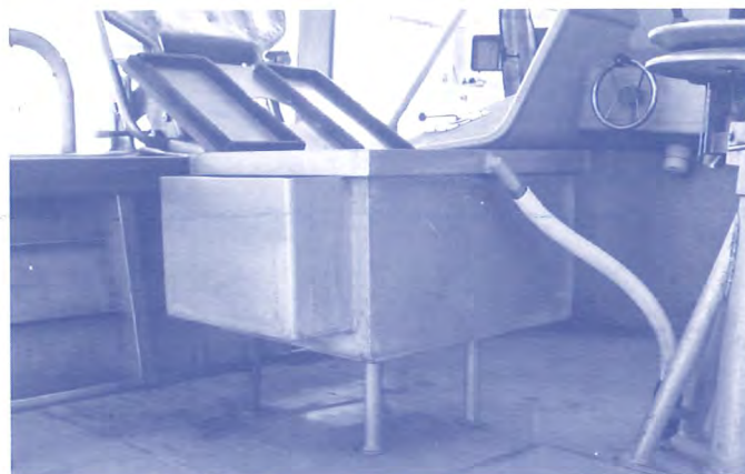
Fig. 2) The cold water stun tank fitted aboard the Shark Raider . For this set up an existing day tank was modified for use as the stun tank.
