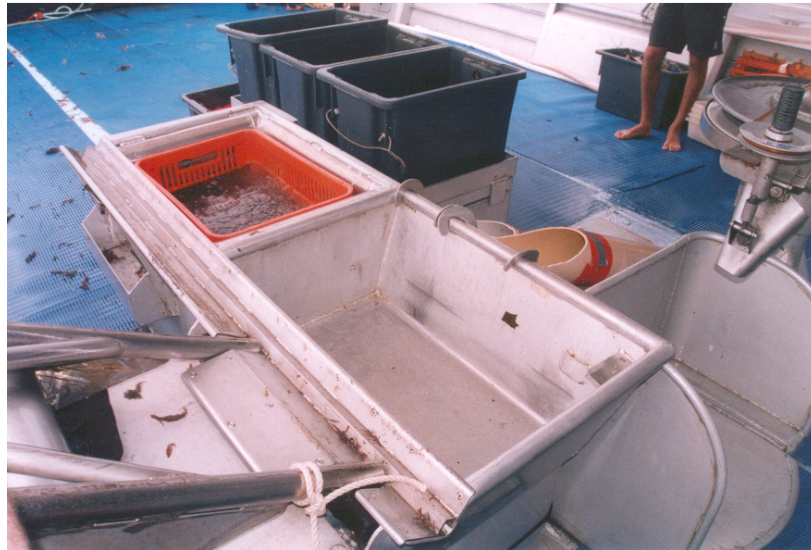
Figure 6) The modified cacka box installed aboard the commercial lobster boat, Windjana. The box consists of a refrigerated seawater-filled stun tank (aft) and a standard aluminium sorting tray (forward). Note the aeration in the stun tank and the 2 chutes (PVC pipes) on the inboard side of the sorting tray that lead down to below deck live tanks.
