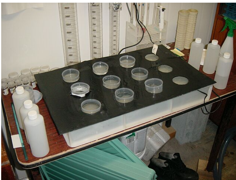
Figure 13) Apparatus for applying combined osmotic and temperature challenge test to larvae. Each cell housed 20 larvae during the test and the cells sat in a controlled temperature water bath.
