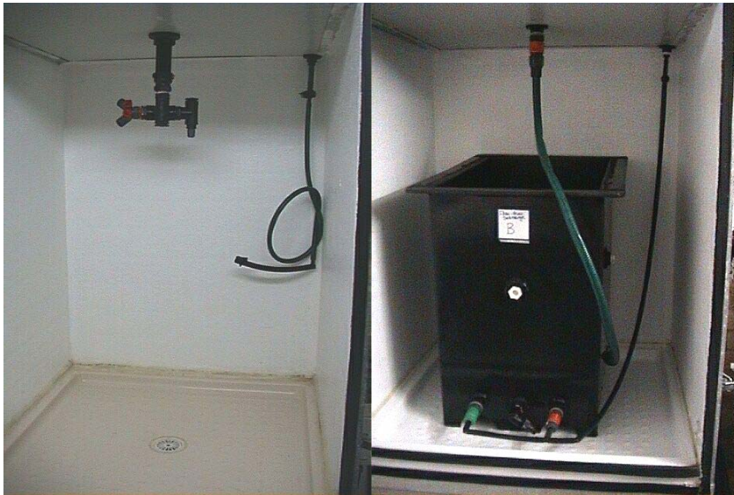
Figure 4) The cubicles used to expose lobsters to different storage environments. For the spray environment (l), baskets of lobsters were placed under ambient seawater sprays. In the submerged treatment (r) baskets of lobsters were submerged in tight-fitting black tanks continuously supplied with seawater and constant aeration.
